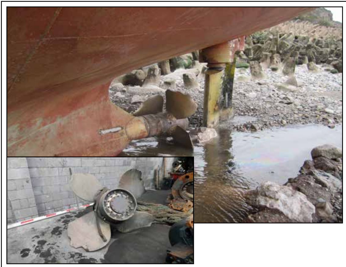
Figure 7: Propeller and rudder damage ( inset: damaged blade tips)
