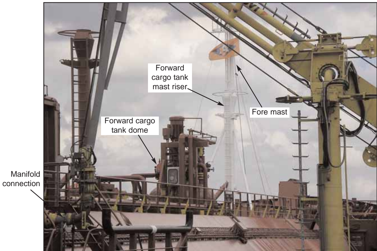
View of mast riser, foremast and forward cargo tank dome
