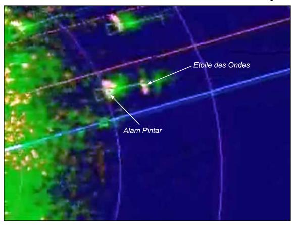
Radar screen shot\* showing Etoile des Ondes fine on Alam Pintar's starboard bow
