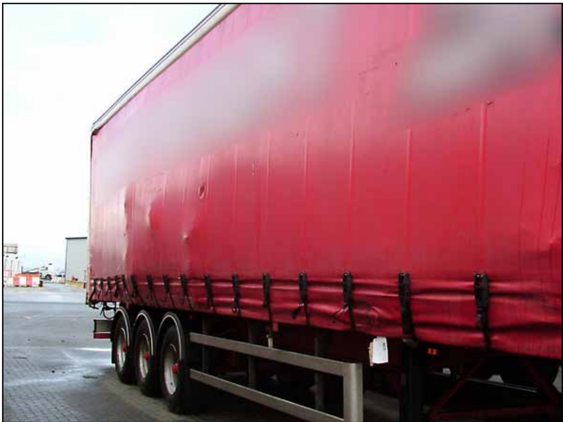
Examples of tautliners with bulging sides prior to shipment
