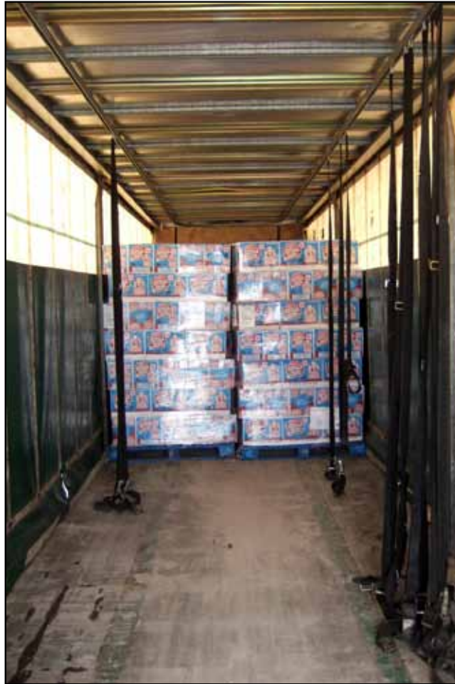
Securing arrangement within a "taughtliner" Note: cargo is not secured down onto the trailer deck
