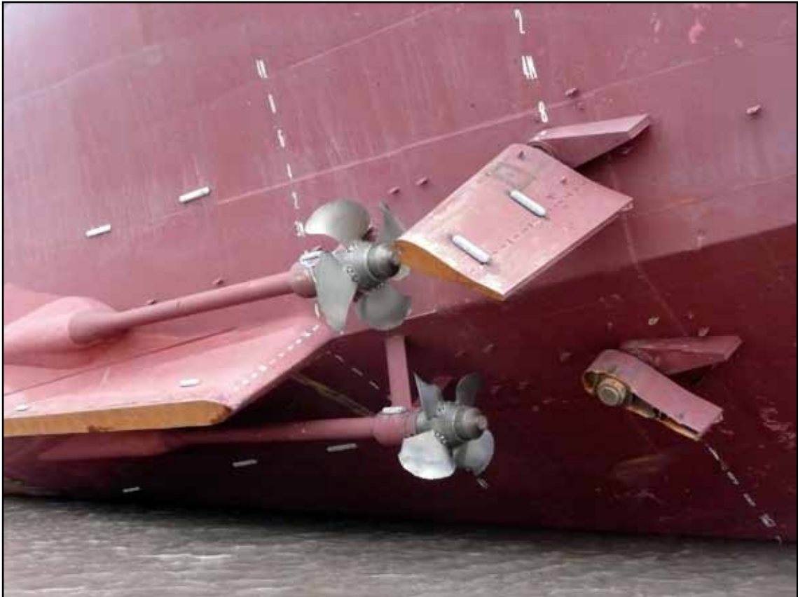
Damage sustained to Riverdance's CPP and starboard rudder
