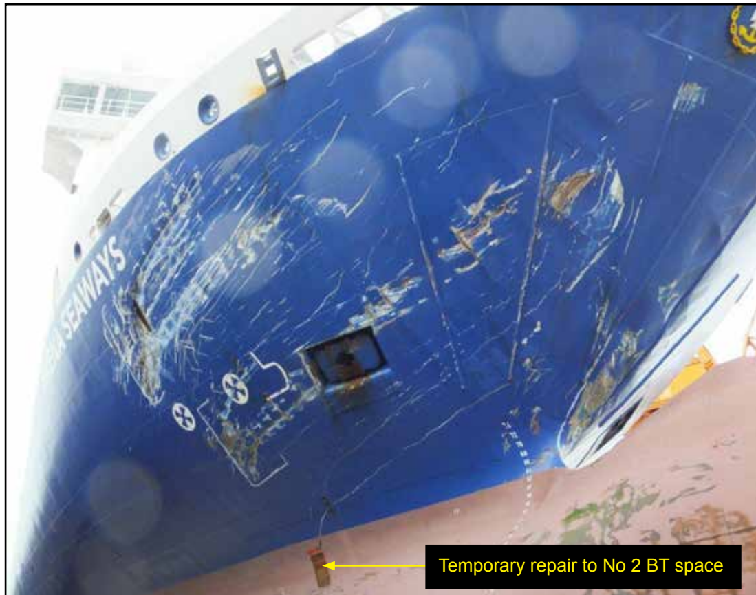
Figure 9a: Starboard bow damage
