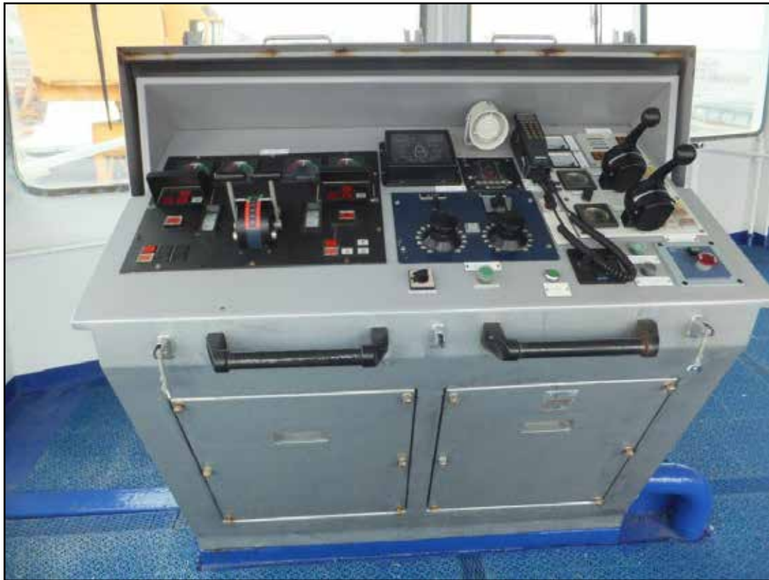
Figure 3: Port bridge wing console
