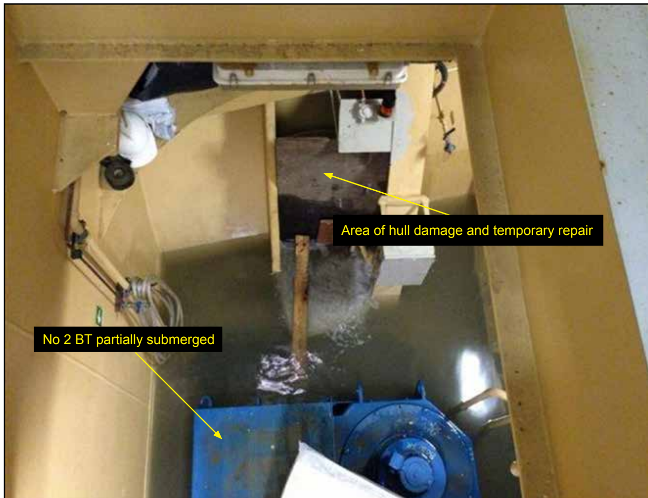
Figure 7: No 2 bow thruster partially submerged
