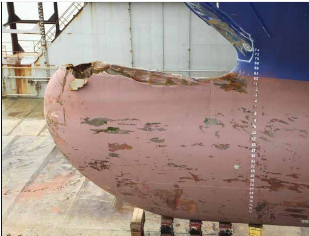
Figure 9b: Damage to upper section of bulbous bow
