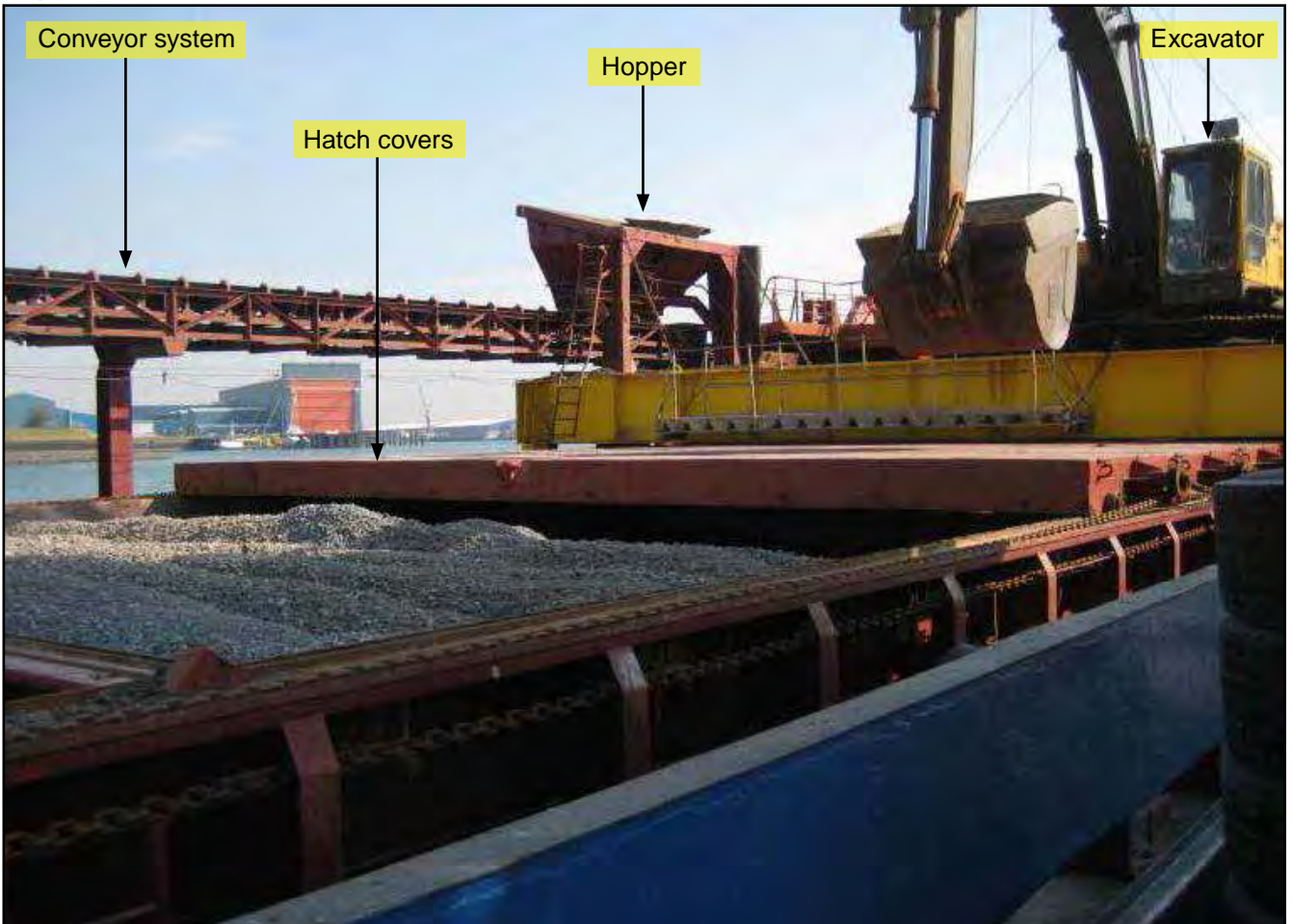
Figure 5: View of open cargo hold hatch covers and cargo hold loaded on a previous occasion
