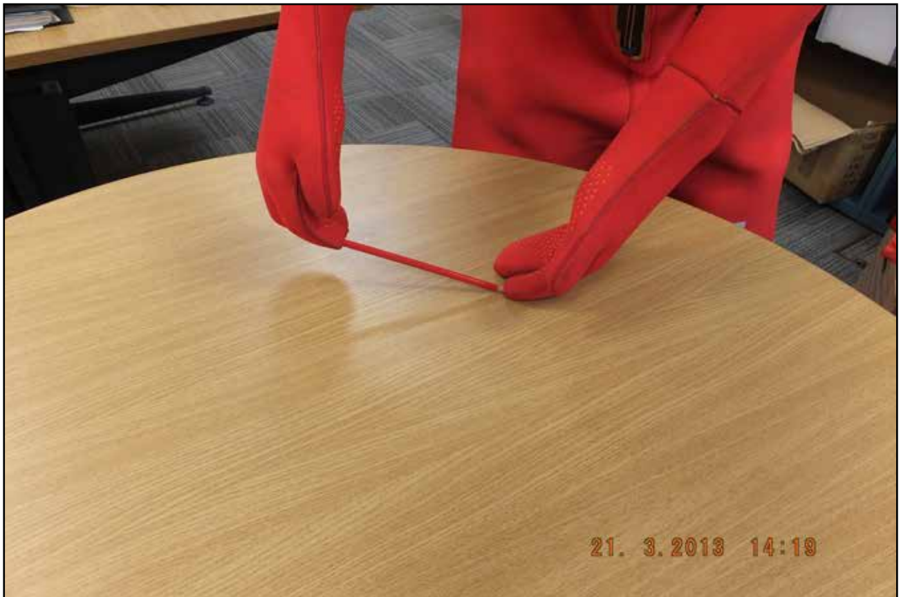
Figures 59a and 59b: Dexterity trial conducted by MAIB using Parkway Imperial immersion suit
