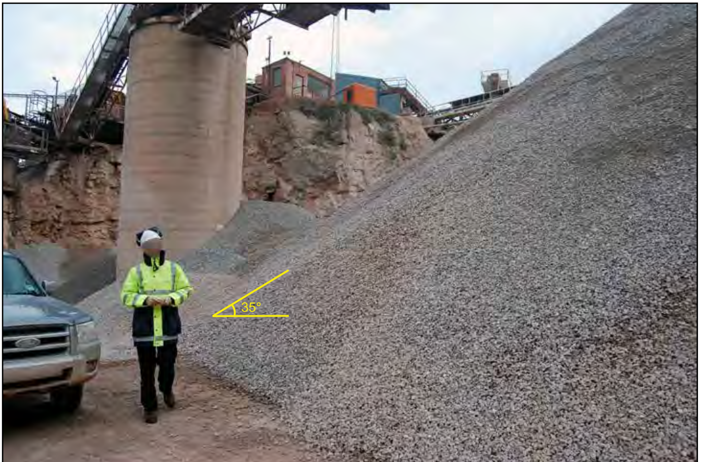
Figure 53: Type 1 limestone stockpile at Raynes Quarry
