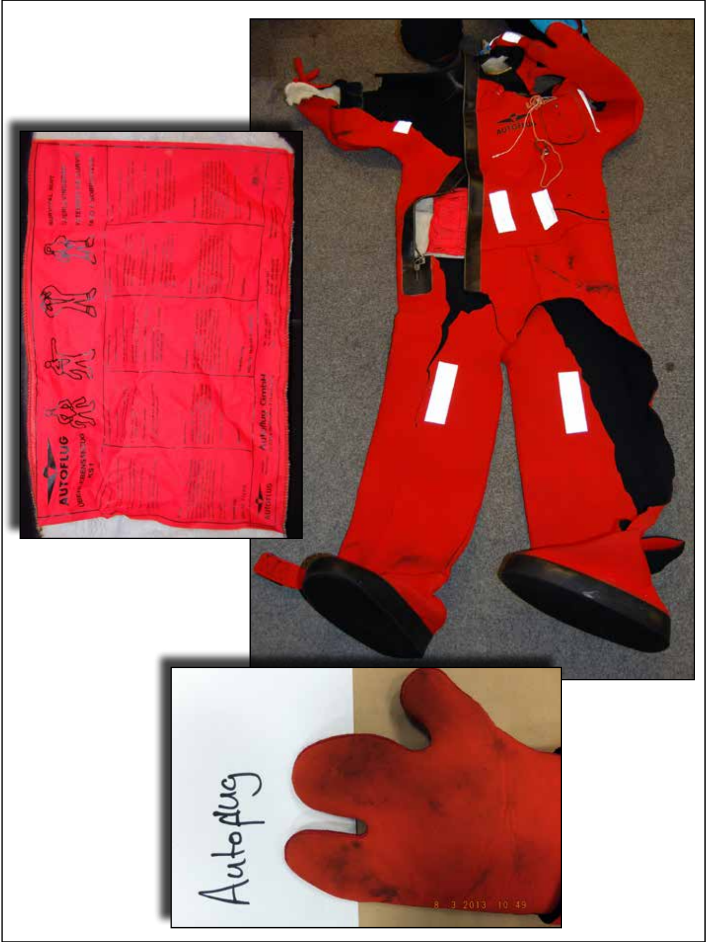
Figure 57: Autoflug K1 immersion suit worn by chief officer, showing label and glove design
