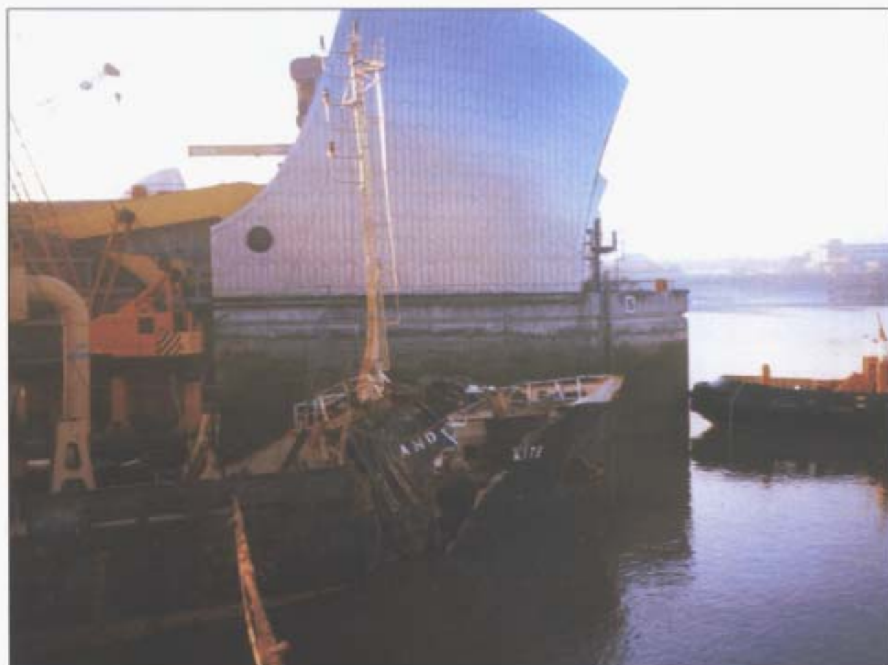
Figure 6: Sand Kite's damaged bow
