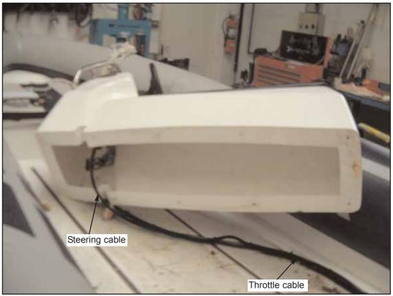
RY5030 console attached by control cables
