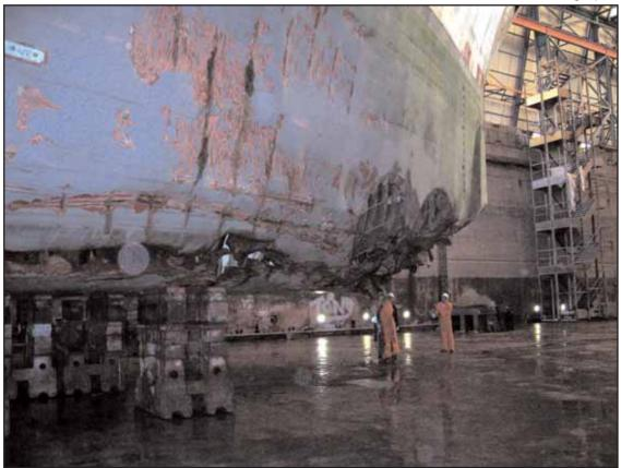
A view of the starboard side looking forward, showing damage to the bow thruster area
