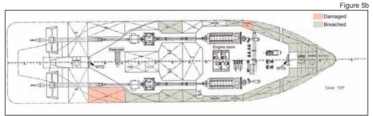
Plan of tank top showing breached and damaged tanks including the intact engine room and pump room
