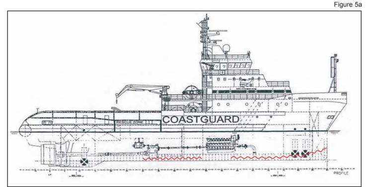
Profile of Anglian Sovereign showing extent of penetration damage on starboard side
