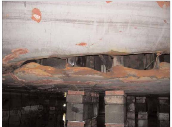
A longitudinal tear in the starboard side shell plating
