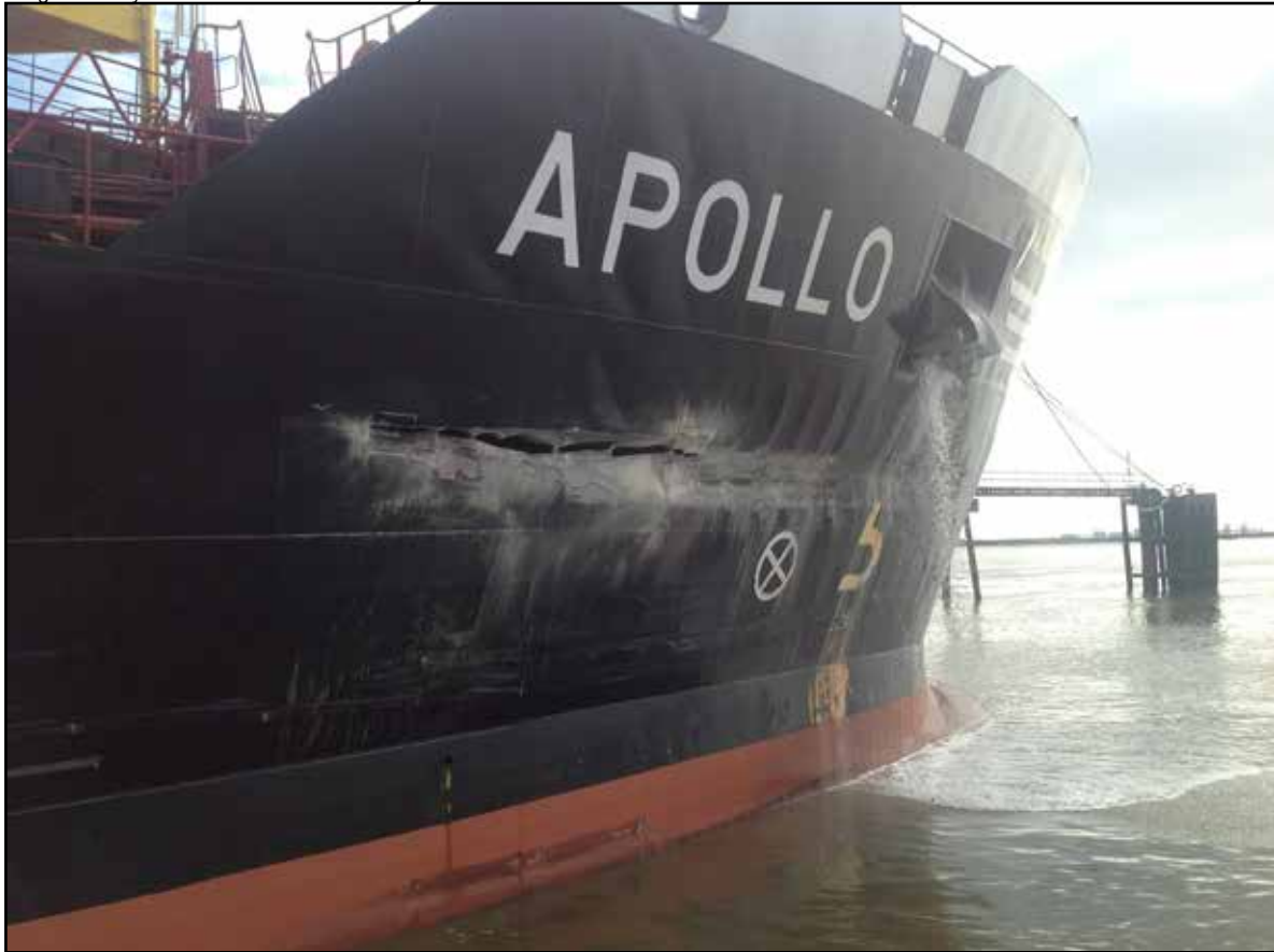
Figure 4: Apollo - damage to shell plating
