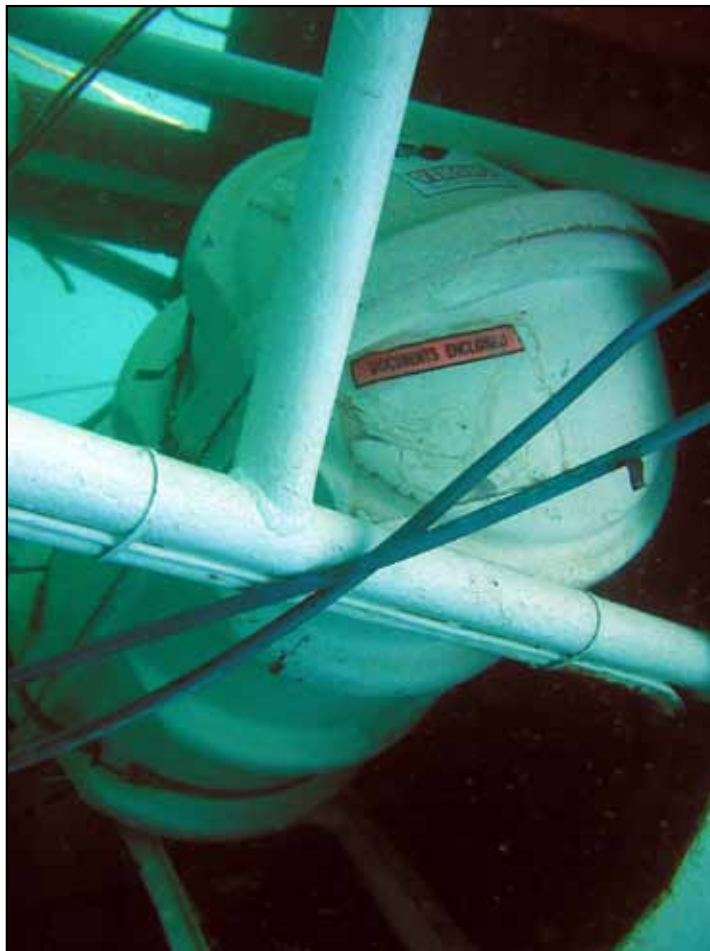
Liferaft fouled in Aquila's superstructure
