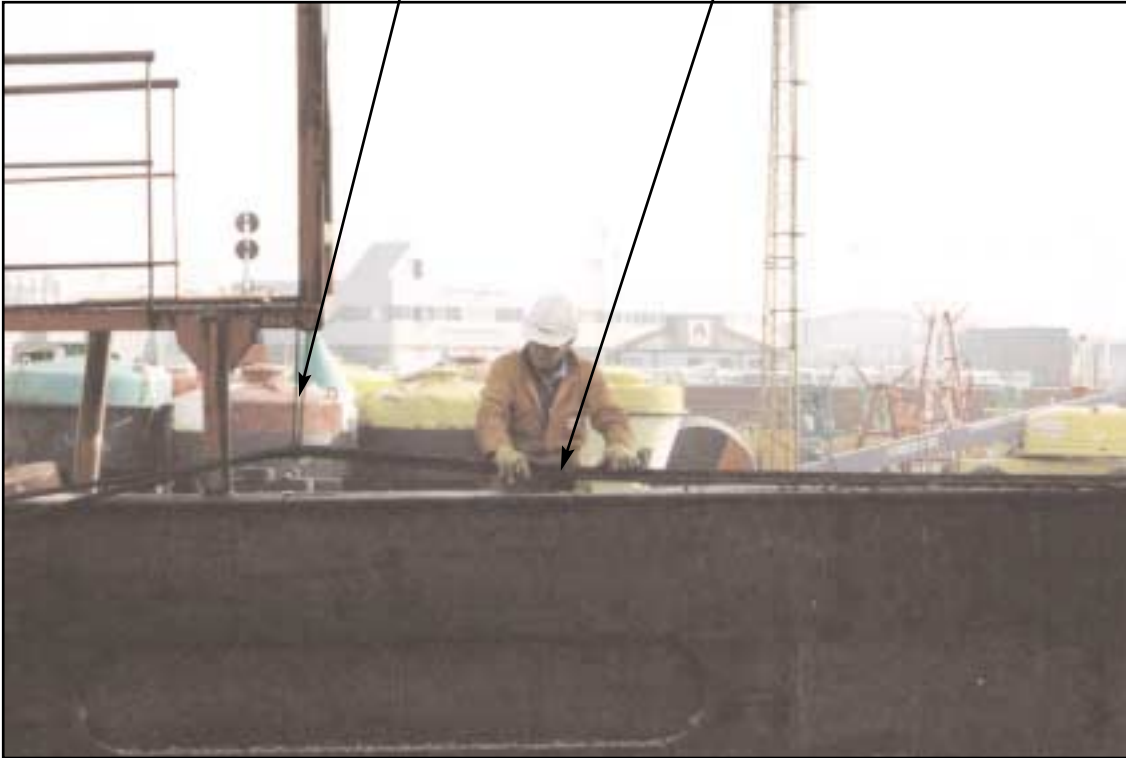
View of port outhaul wire positioned on coaming behind forward retaining hook
