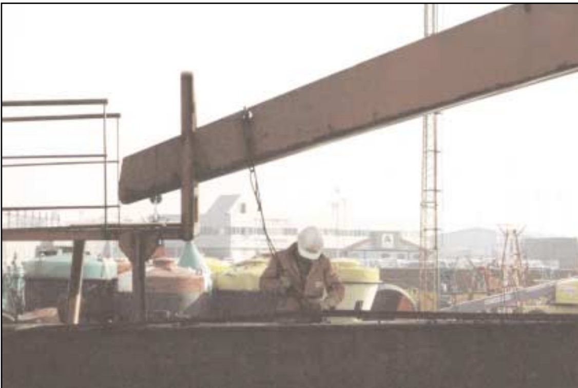
View of lifting strop being released from outhaul wire. Loading chute in stowed position.
