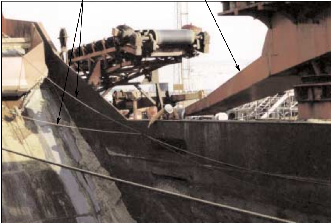
View of port outhaul wire being manhandled on to aft retaining hook
