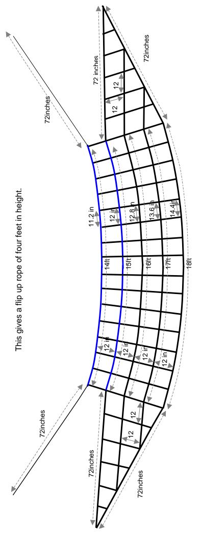
Vertical ropes at 11.2 inch spaces **TOP ROPE LENGTH 14 FEET**
