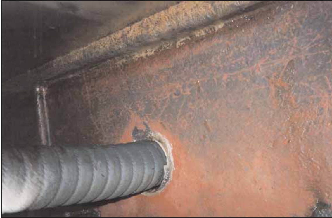
Penetration of aft bulkhead by exhaust hose
