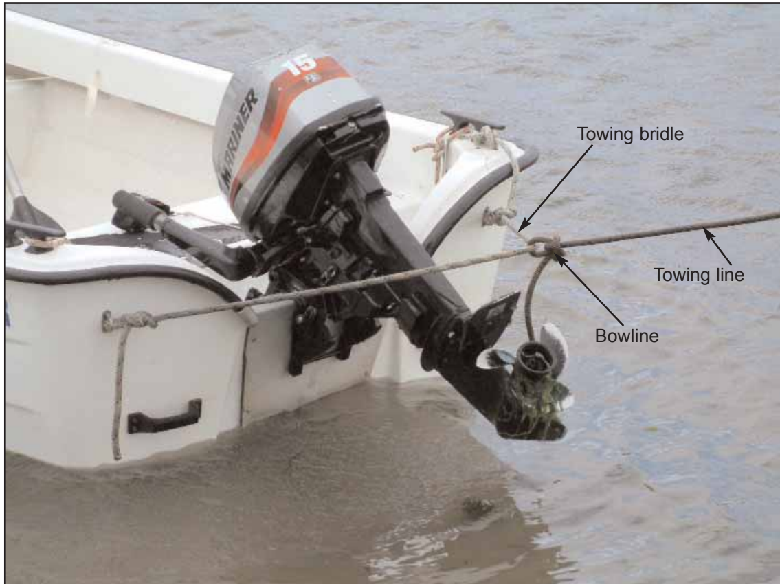
Safety boat bridle and towing line arrangement
