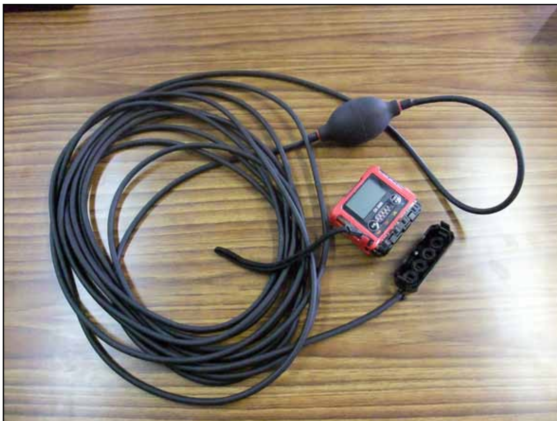
Riken Keiki GX-2009 (Ex Type A) Personal Gas Monitor, with aspirator and 10m sampling hose extension arrangement
