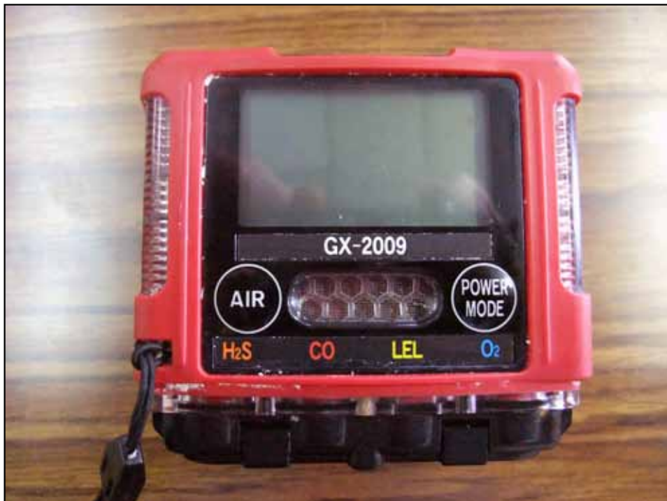
Riken Keiki GX-2009 (Ex Type A) Personal Gas Monitor
