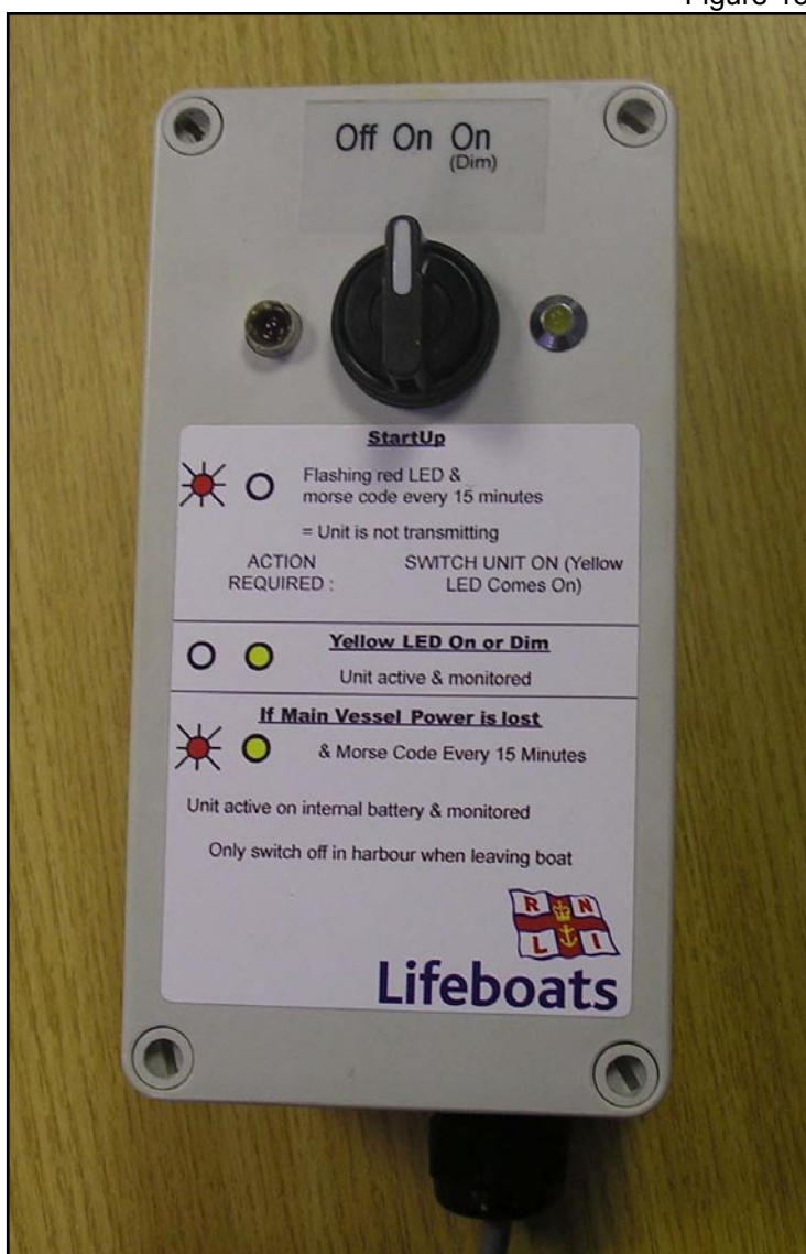
CPRS control unit switched ON (Sample unit)
