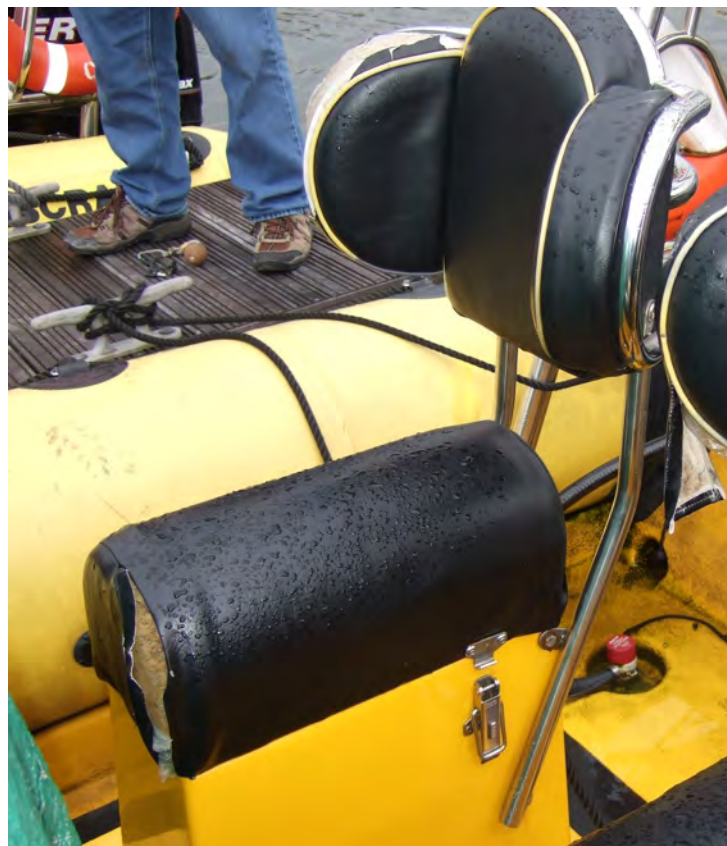
Figure 5. An example of wear-and-tear on a RIB seat, demonstrating a lack of maintenance, which accelerates the degradation of the seat cushion.
