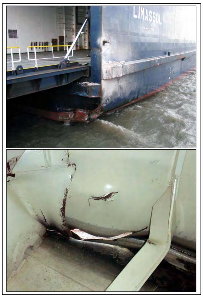
Figure 8: Damage to Clipper Point
