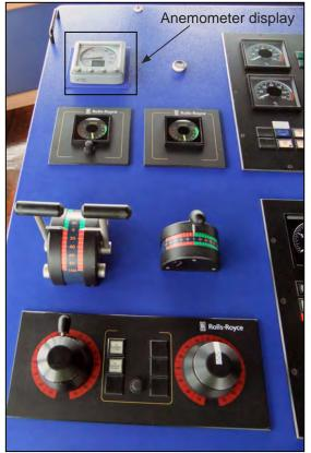
Figure 13: Bridge wing wind indicator
