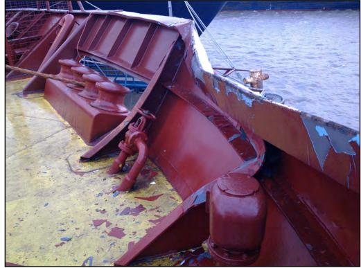
Figure 10: Damage to Scotia Seaways
