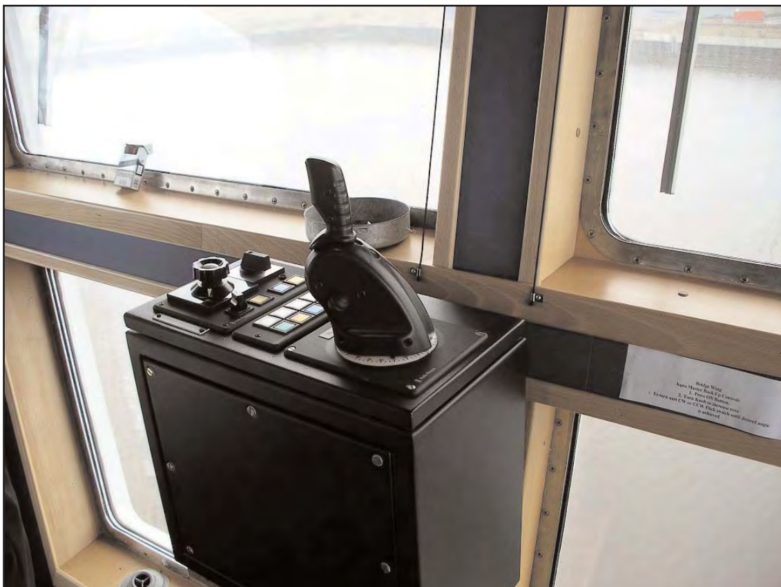
The second bridge wing thruster control handset
