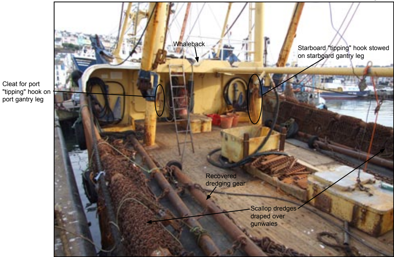
Main deck looking forward towards whaleback
