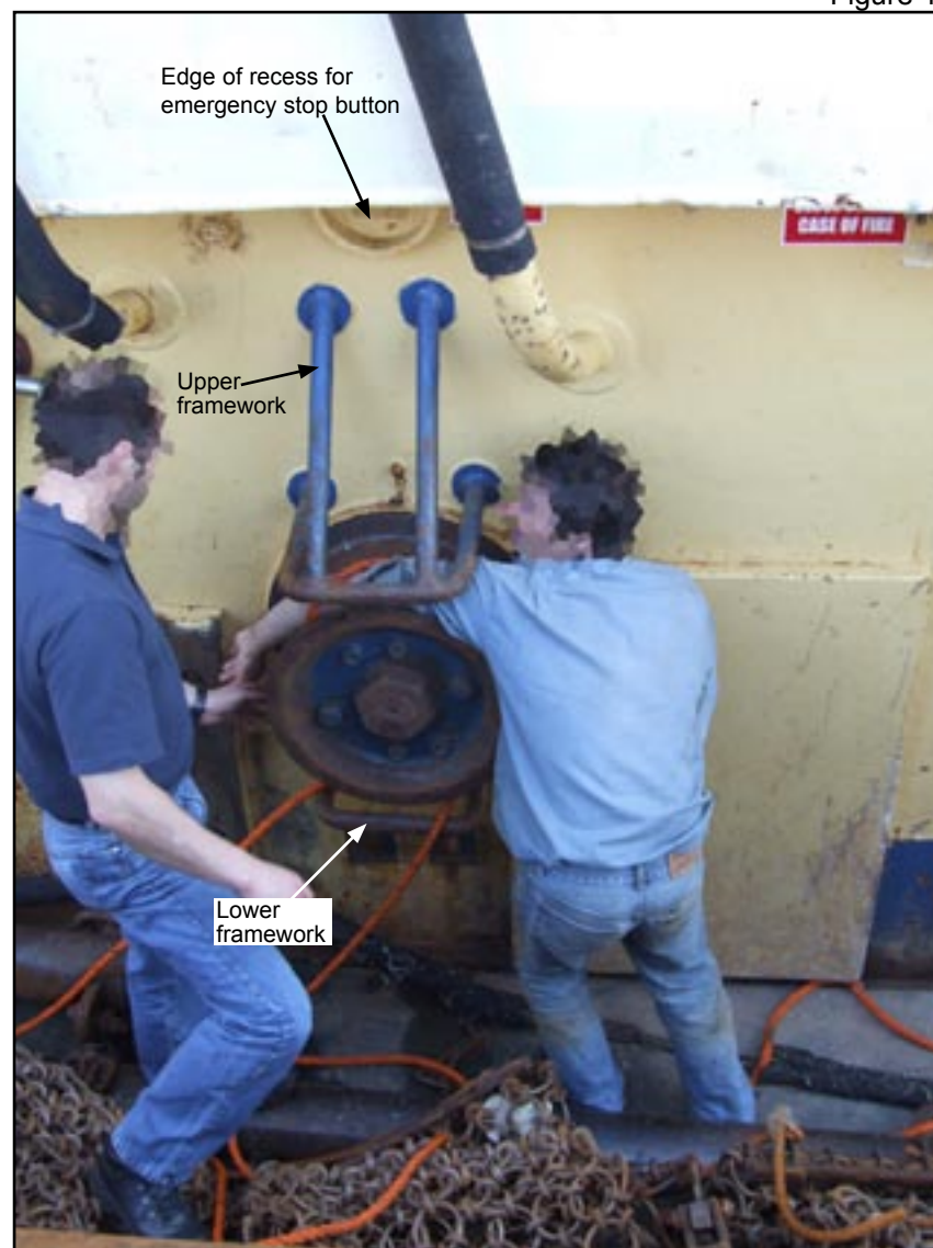
Demonstration of “as-found” position of deckhand, trapped in whipping drum
