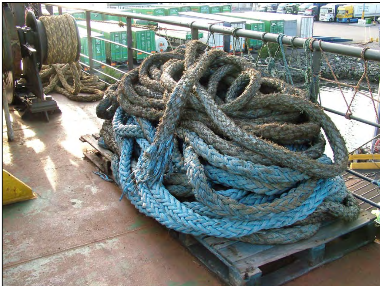
Parted stern line in normal storage position
