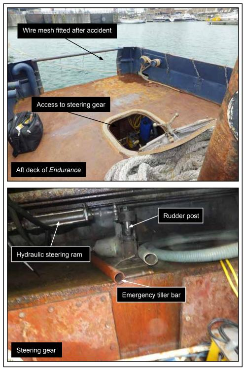
Figure 26: Endurance's steering gear arrangement
