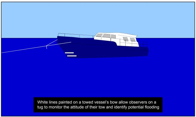
Figure 27: Example of the bow markings recommended in the SCV Code for unmanned towed vessels
