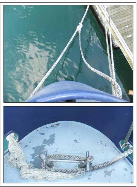
Figure 24: Tow rope securing arrangement reconstructed on *Sirius M*'s foredeck
