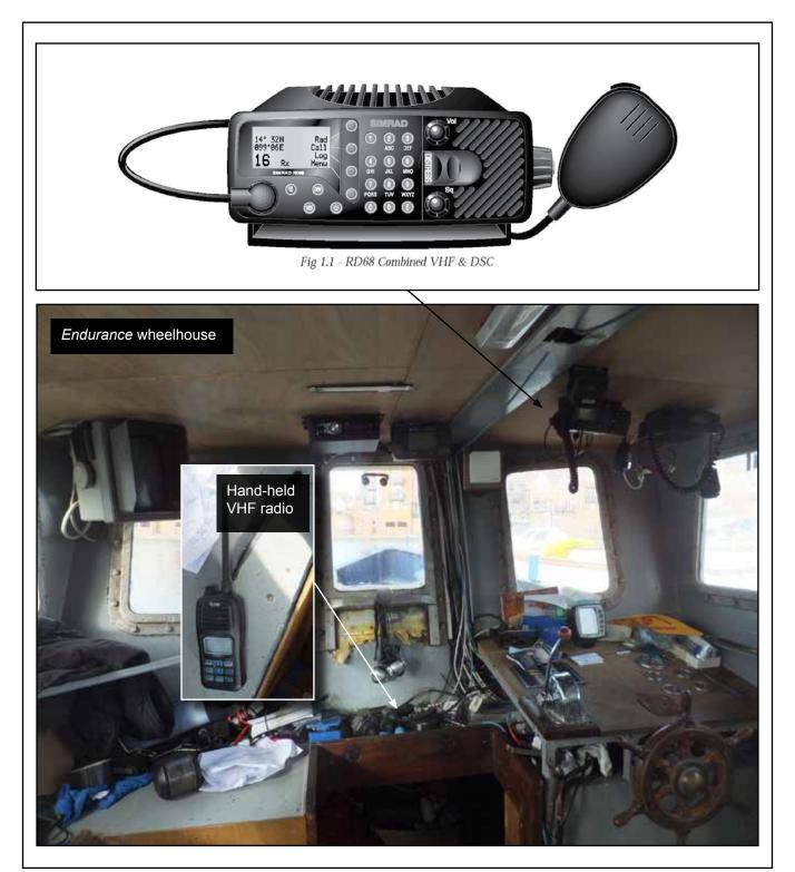
Figure 18: Combined VHF and DSC radio fitted on board Endurance
