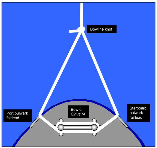
Figure 22: Towline securing arrangement
