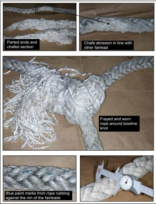
Figure 25: Tow rope chafe marks and frayed ends, and fraying at the bowline knot used to form the towing eye
