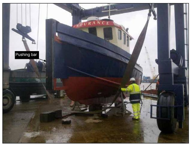
Figure 16: Endurance out of the water in 2012 - pushing bar fitted
