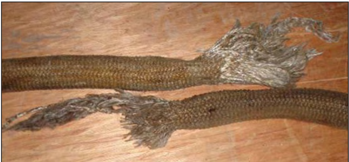
Tow rope failure
