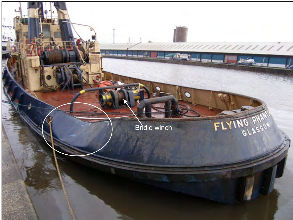
Aft deck showing parbuckle damage and location of bridle winch
