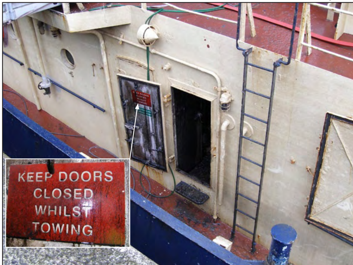
Engine room watertight door
