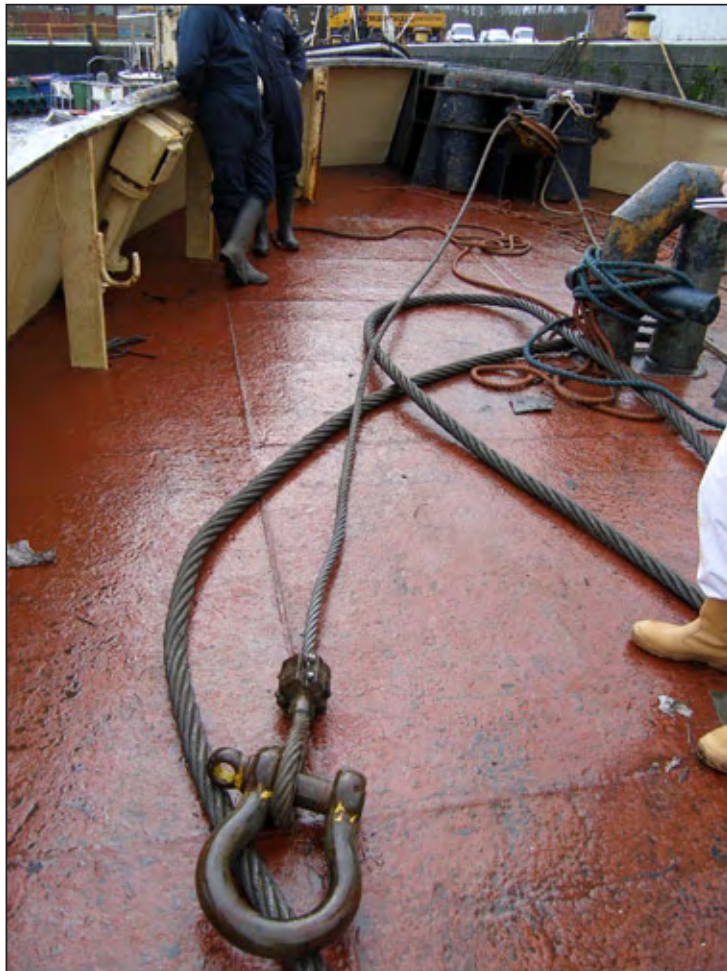
Swivel fairlead on transom, bridle wire and bow shackle
