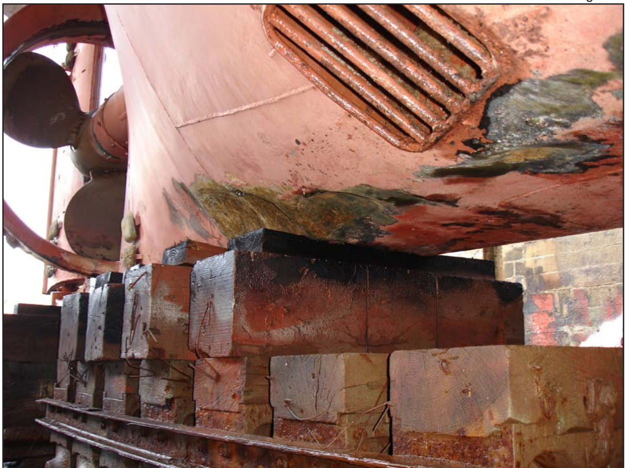
Photograph of damage to hull plating
