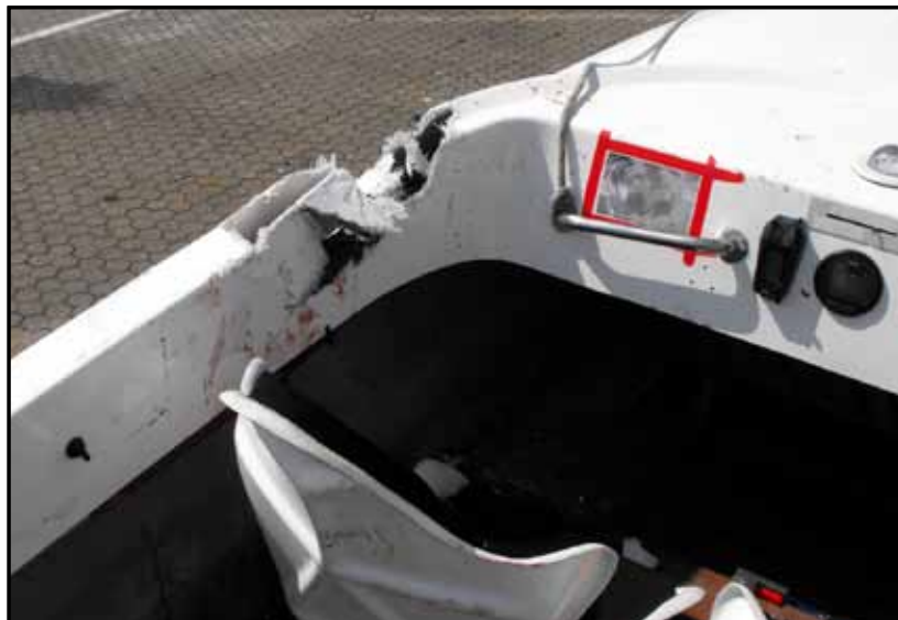
Impact damage to port side cockpit coaming
