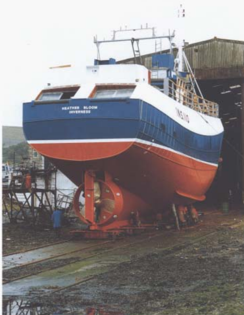
HEATHER BLOOM near completion, showing the transom openings and doors
