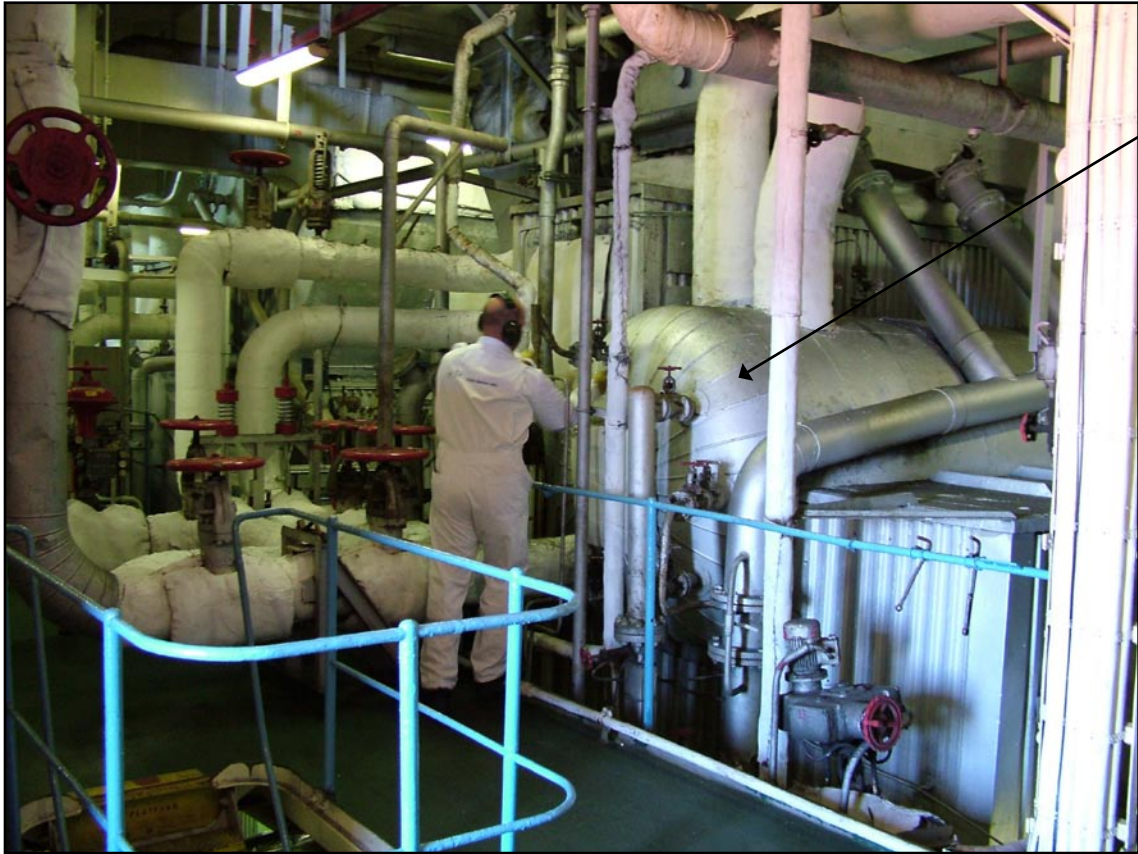
Forward view of the starboard boiler steam drum top plate level
