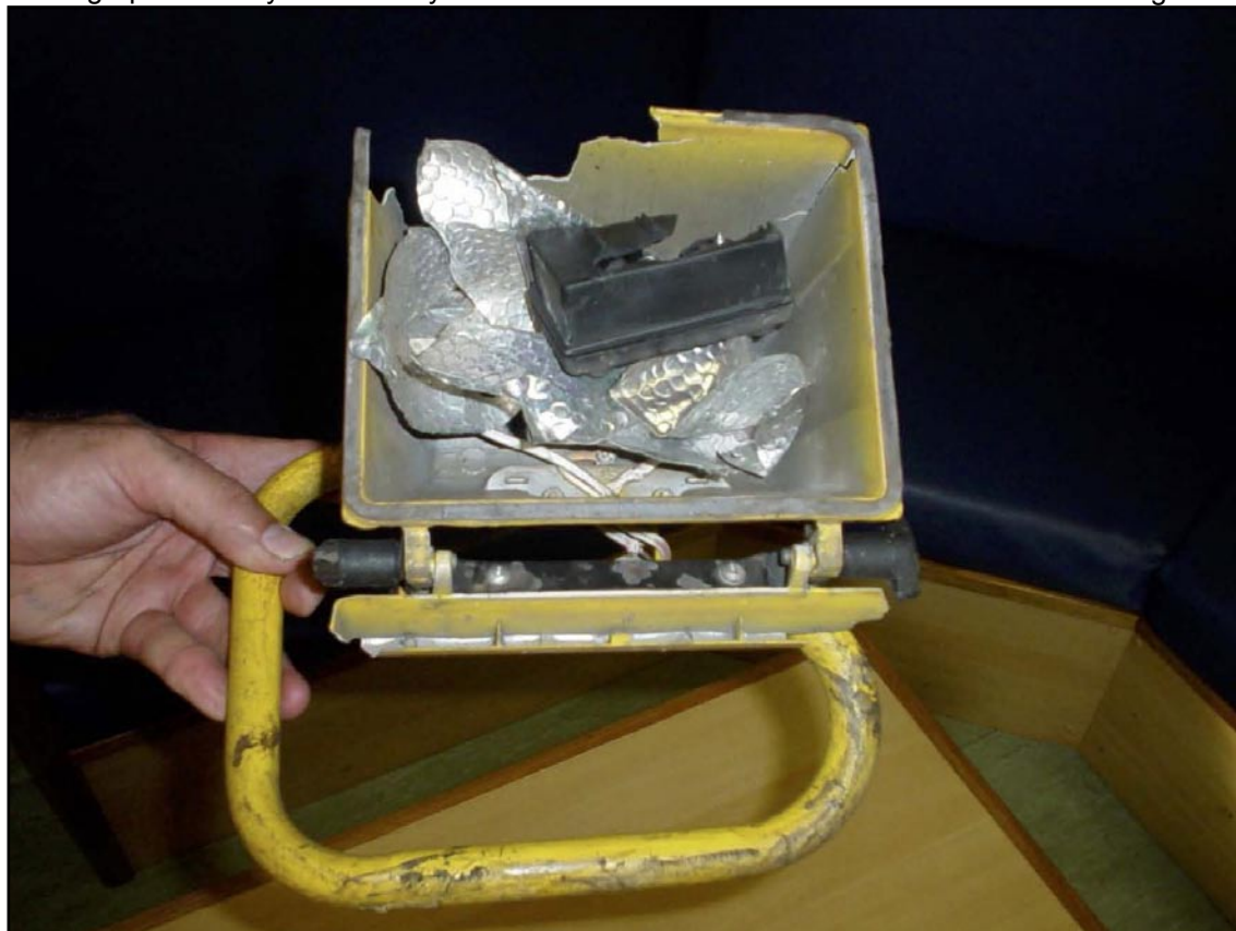
Damaged halogen lamp
