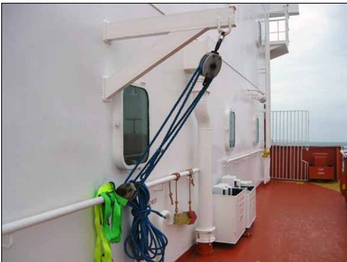
Gantry arrangement used for rescue
