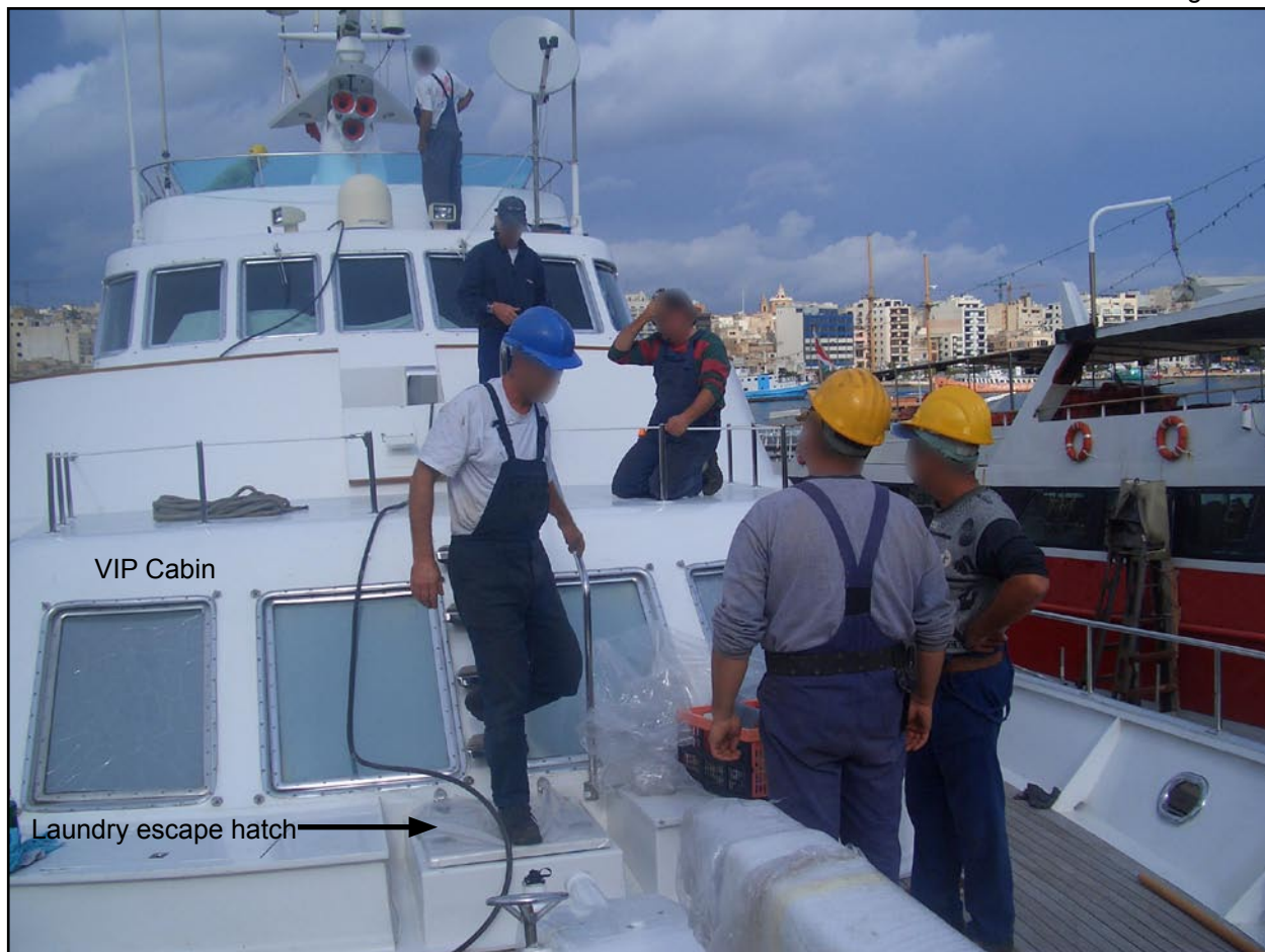
Foredeck, escape hatch and VIP cabin
