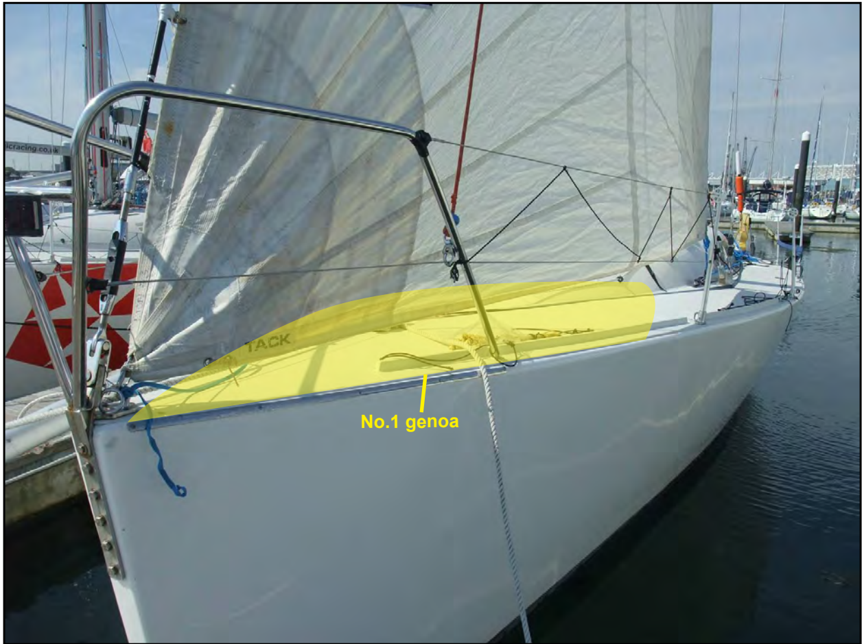
Figure 3: Position of the lashed No.1 genoa
