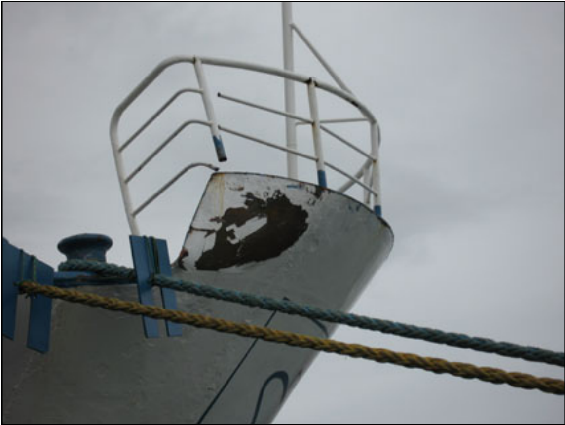
Damage to starboard bow of Logos II
