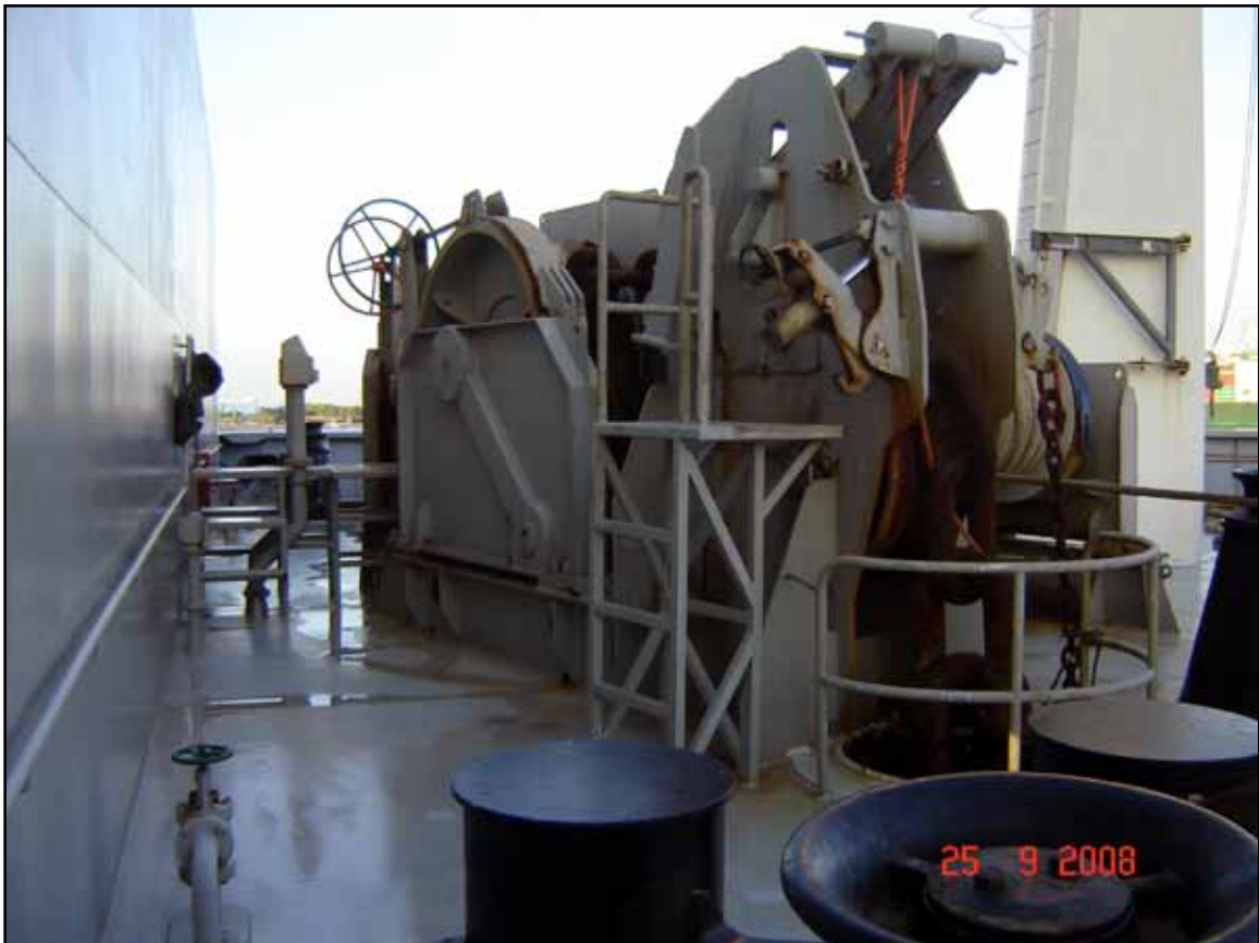
The starboard anchor windlass
