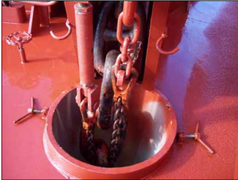
Chain lashing arrangement
