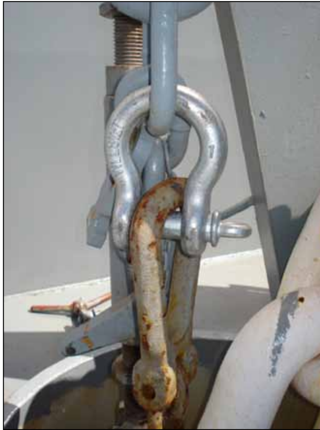
Safmarine Nyassa's starboard anchor Senhouse slip sheared tapered securing pin bow shackle replaced arrangement
