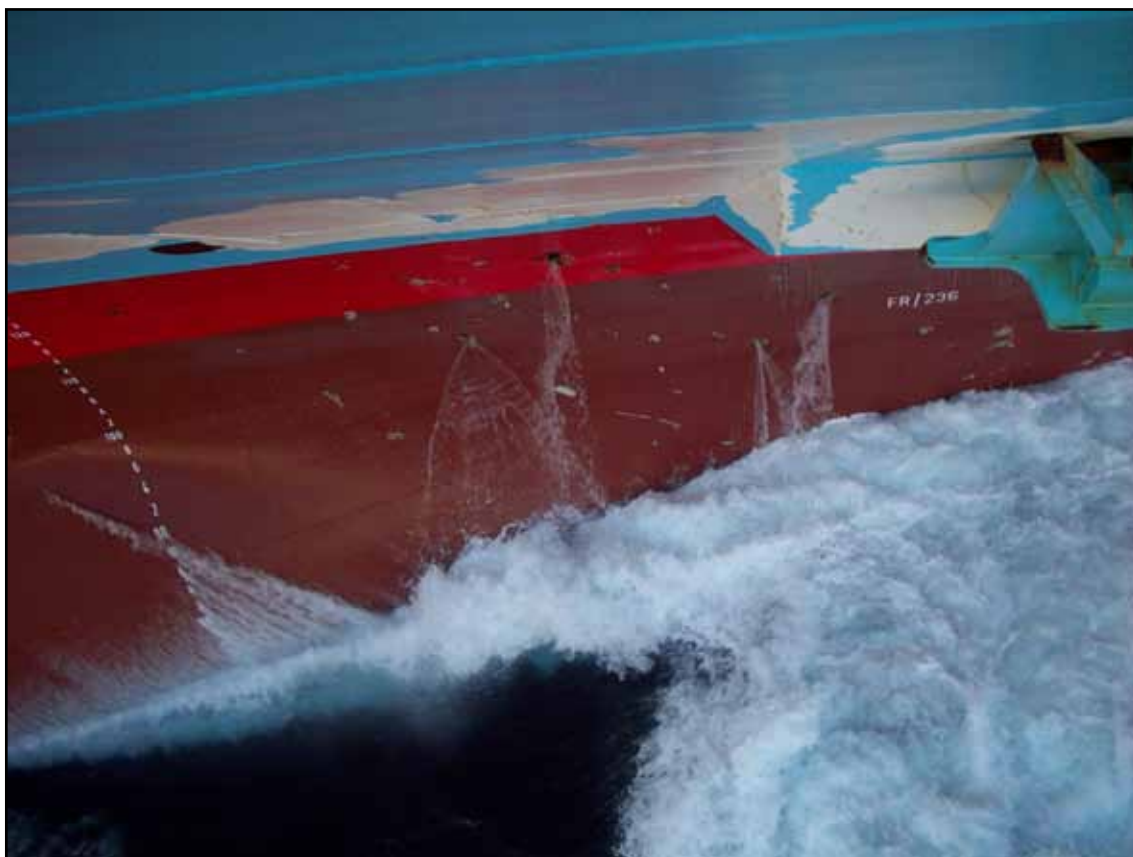
Damage to the port side of the hull seen from the forecastle
