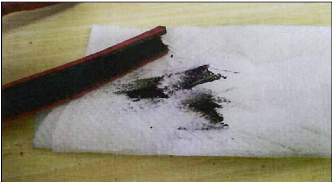
Carbon deposits on the inside of an acetylene hose - typical indications of a flashback
