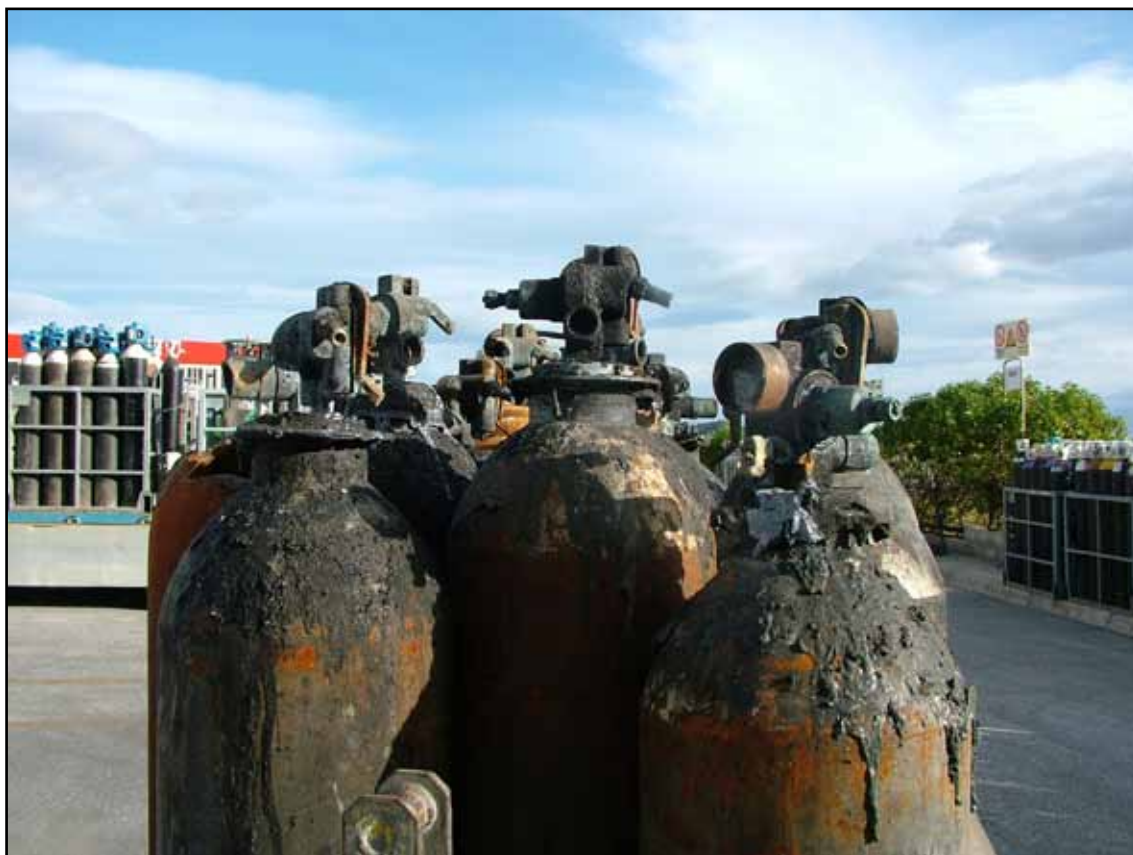
Fire damaged oxygen bottles
