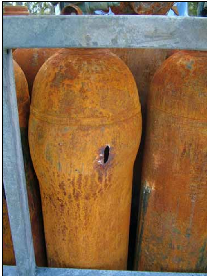
Distorted acetylene bottles
