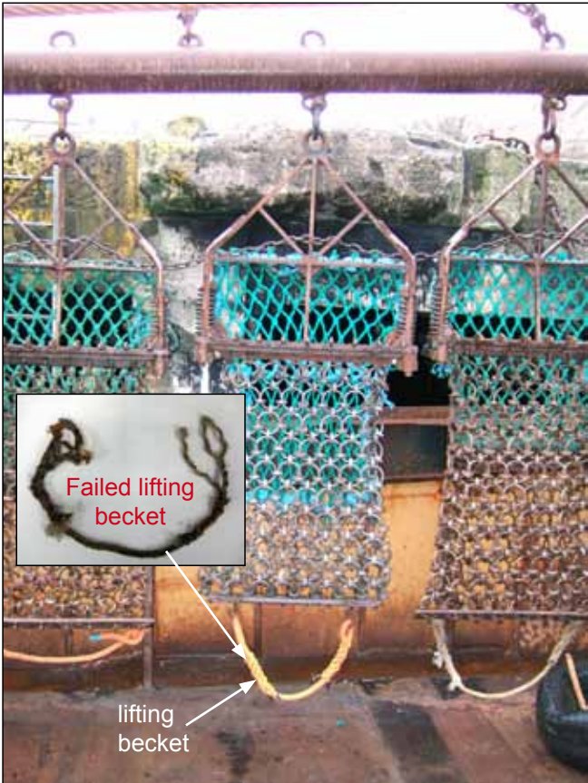
Dredge bags and the parted lifting becket
