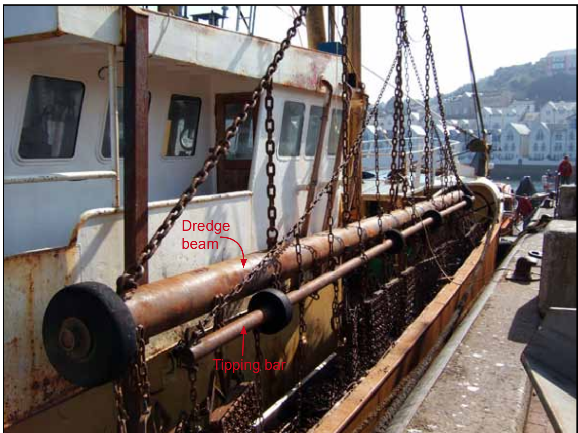
Fitted 'tipping bar' arrangement
