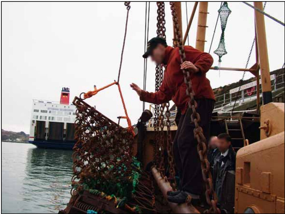
Simulation by deckhand - shaking the dredge bag
