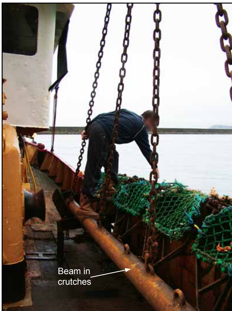
Simulation by deckhand - snaring the lifting becket
