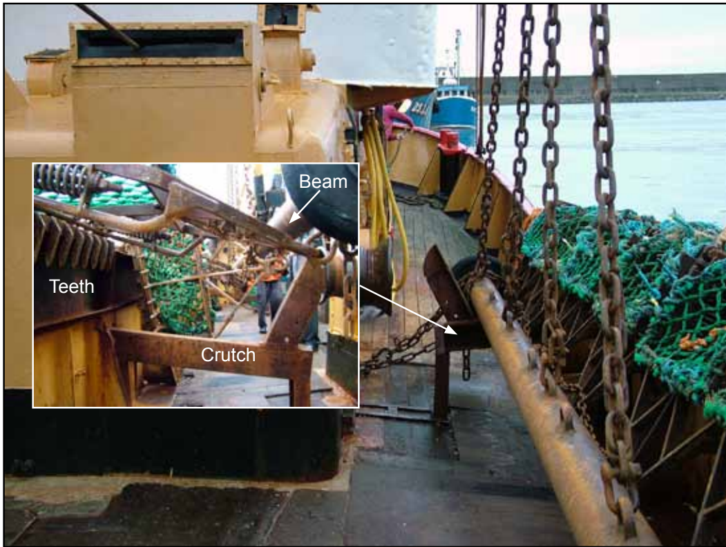
Position of dredge beam when resting on crutches
