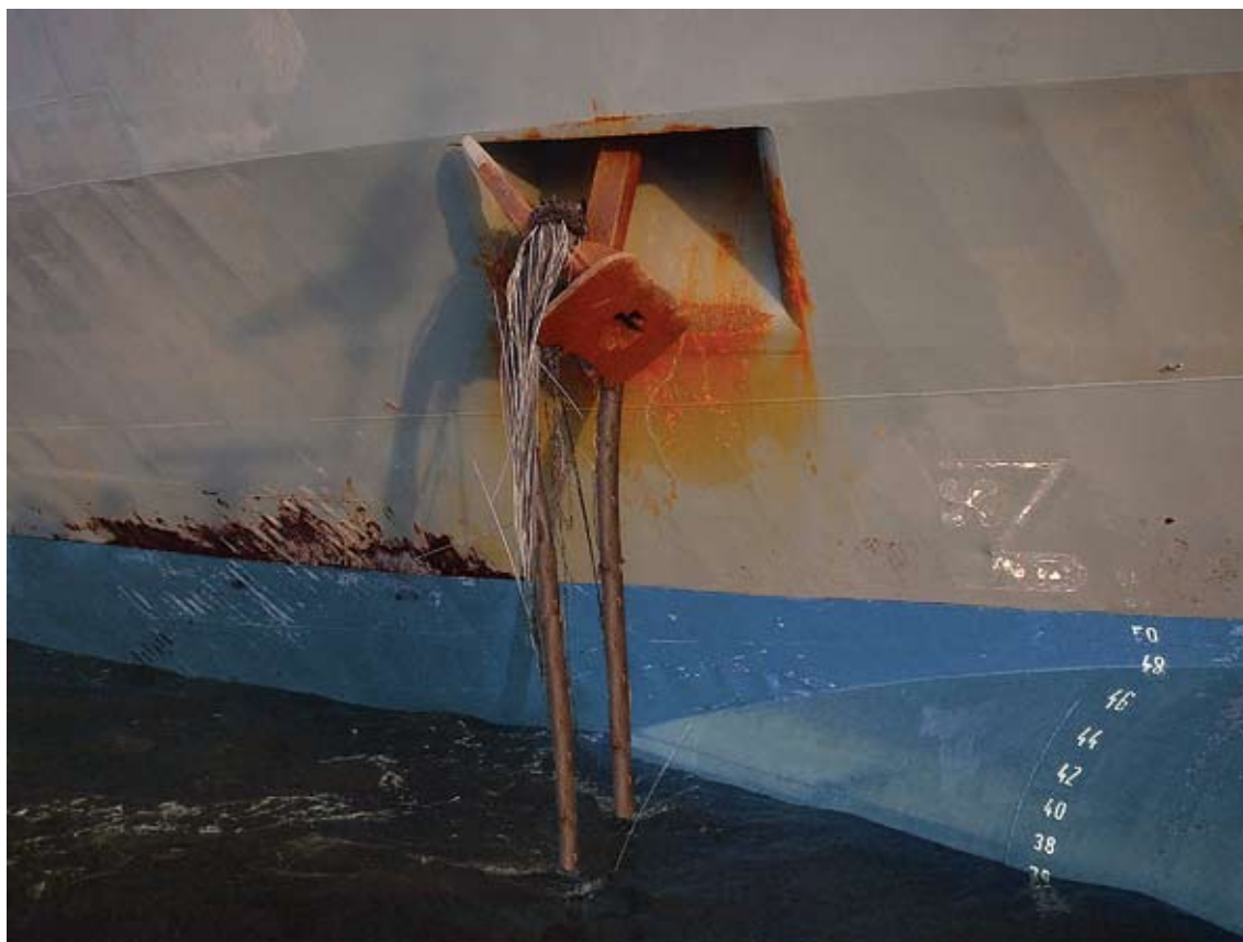
Vessel's anchor, fouled with a power cable
