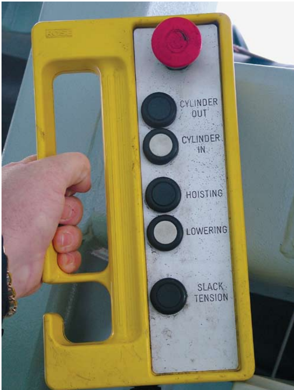
Figure 3 – FRC winch controller
