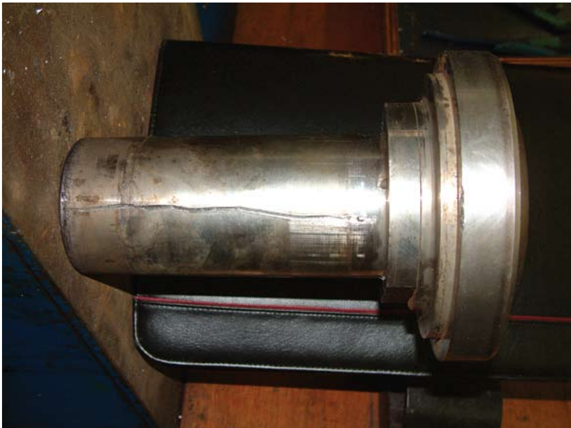
Scoring damage on valve disc body
