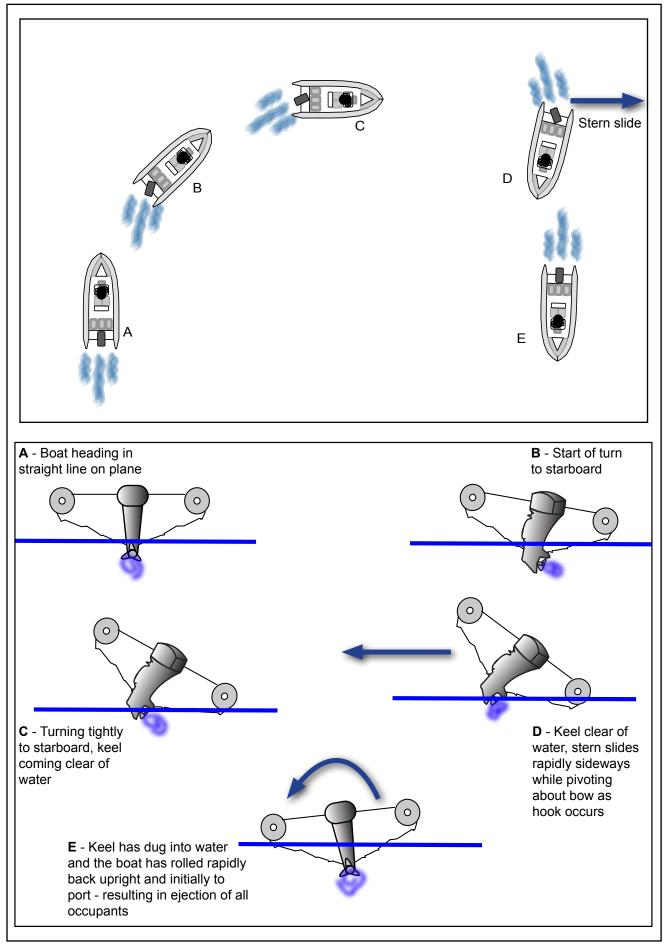
Figure 12: Diagram showing a hook during a turn
