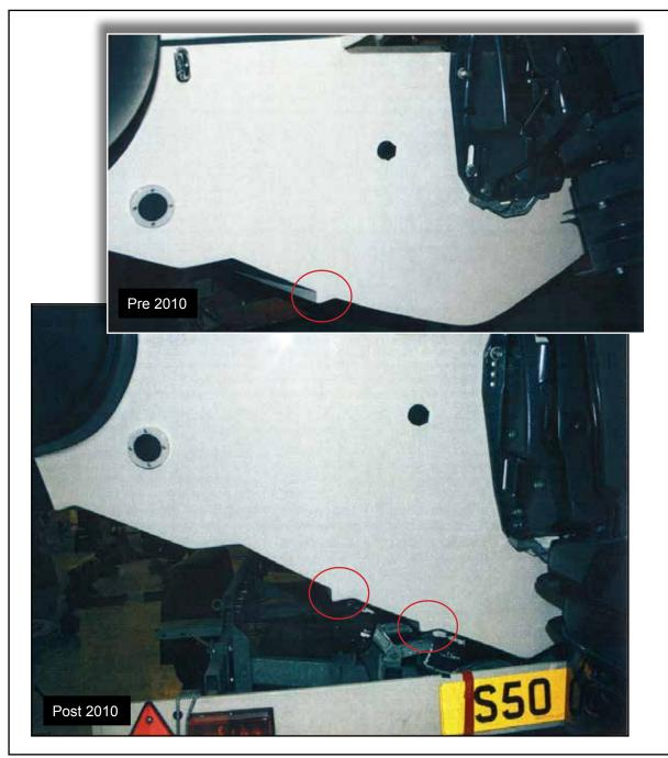
Figure 7: Hull design changes made to Cobra RIBs by manufacturer in 2010
