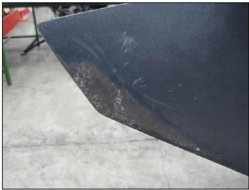
Figure 8: Milly - abrasion mark found on engine skeg post-accident
