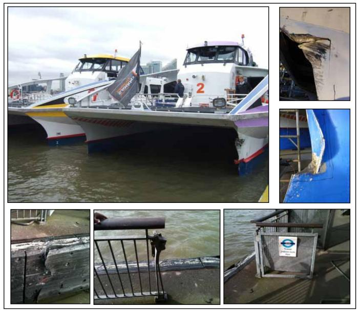
Figure 12: Damage caused by the contact
