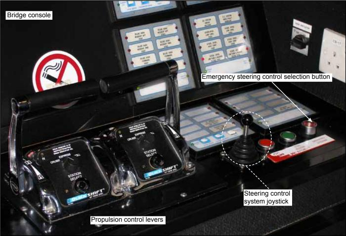
Figure 2: Steering control system joystick
