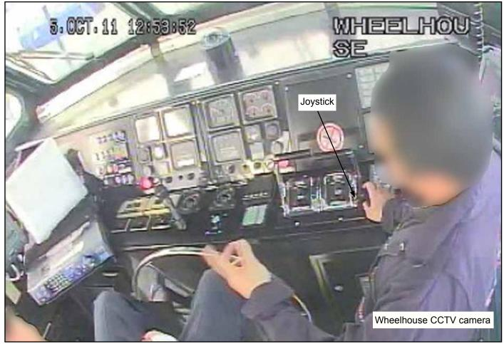
Figure 3: Service engineer investigating the reported steering joystick fault (CCTV time local + 3 minutes)
