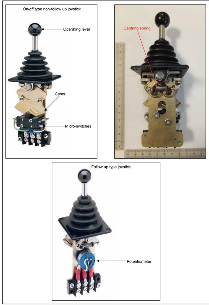
Figure 16: Kobelt model 7165 compact single axis joystick
