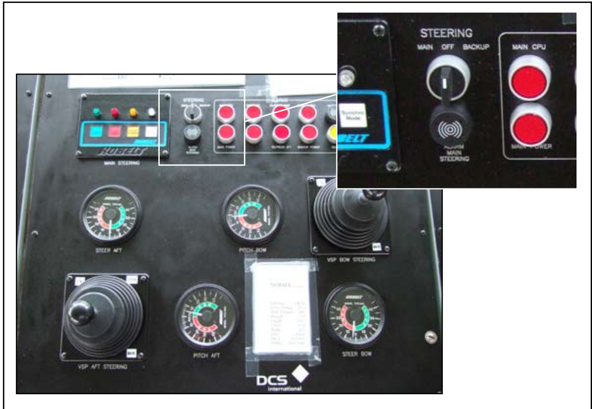
Propulsion and steering control panel
