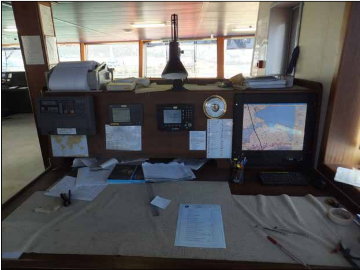
Figure 7: ECDIS planning terminal
