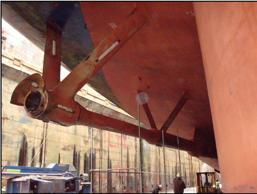
Port side missing CP propeller and hub
