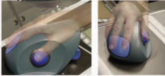
The operating control has a convenient thumb-operated trackball, with right and left click buttons on the front.
