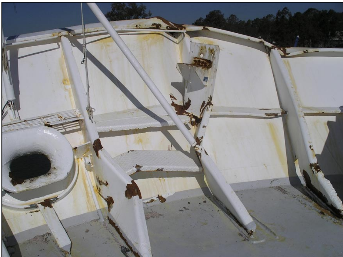
Damage to forecabin bulwark
