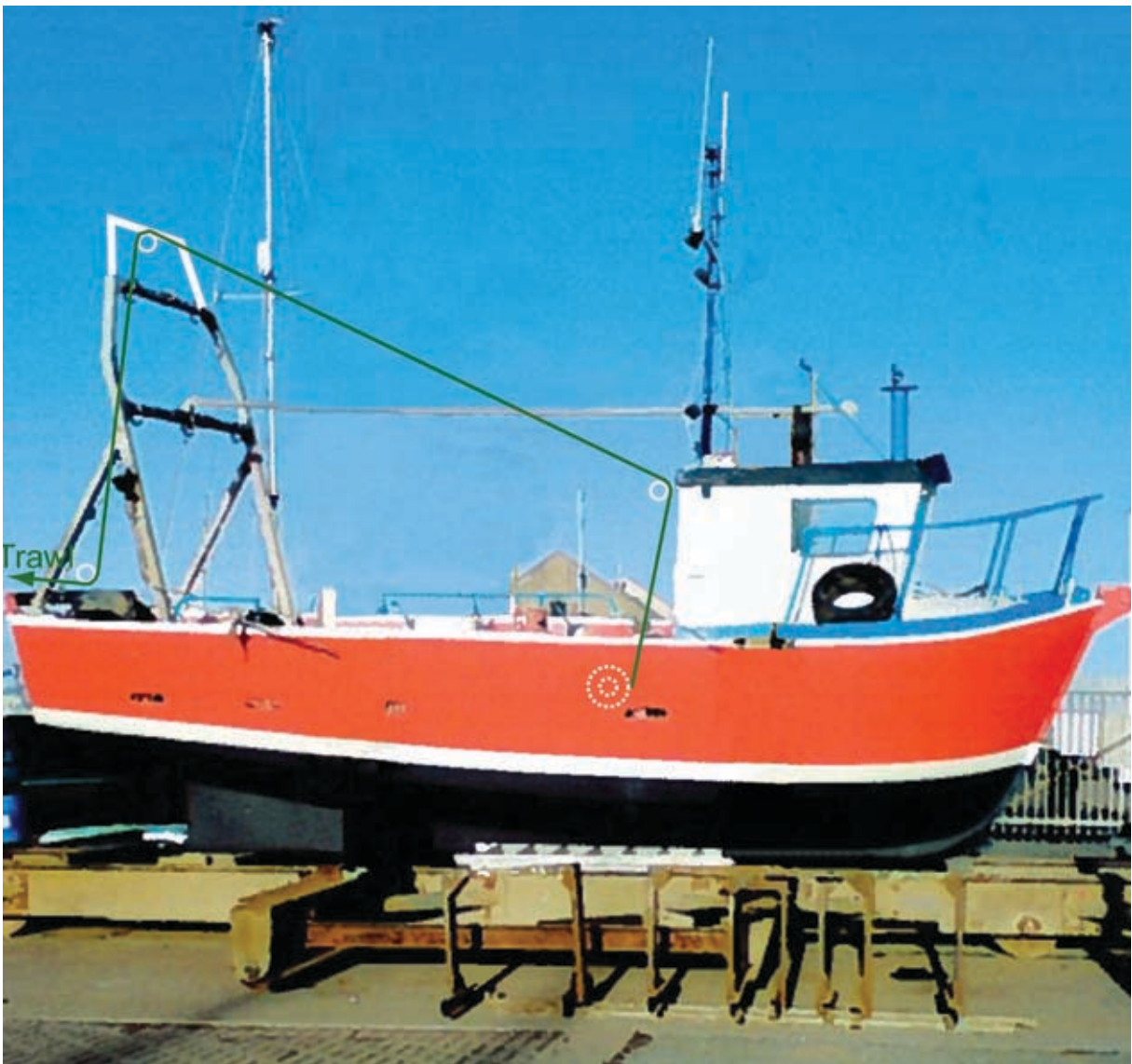
Vessel with illustration of trawler assembly
