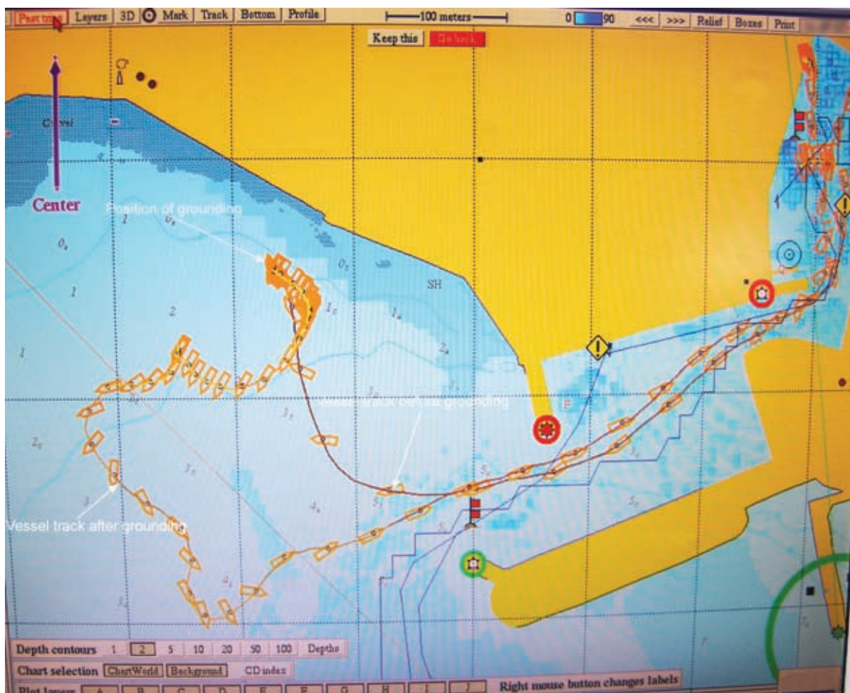
Vessel's track – recorded from electronic chart plotter
