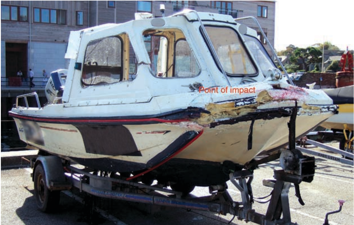
Figure 3: Damage to bow of the dory
