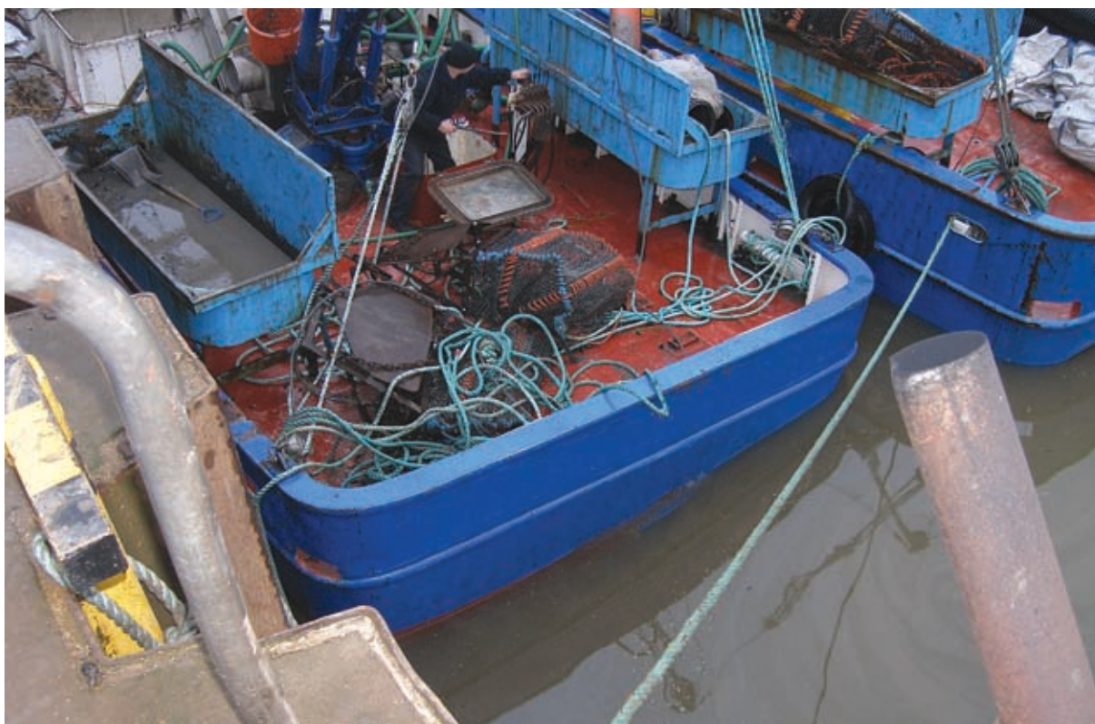
Figure 2: View of stern showing limited freeboard
