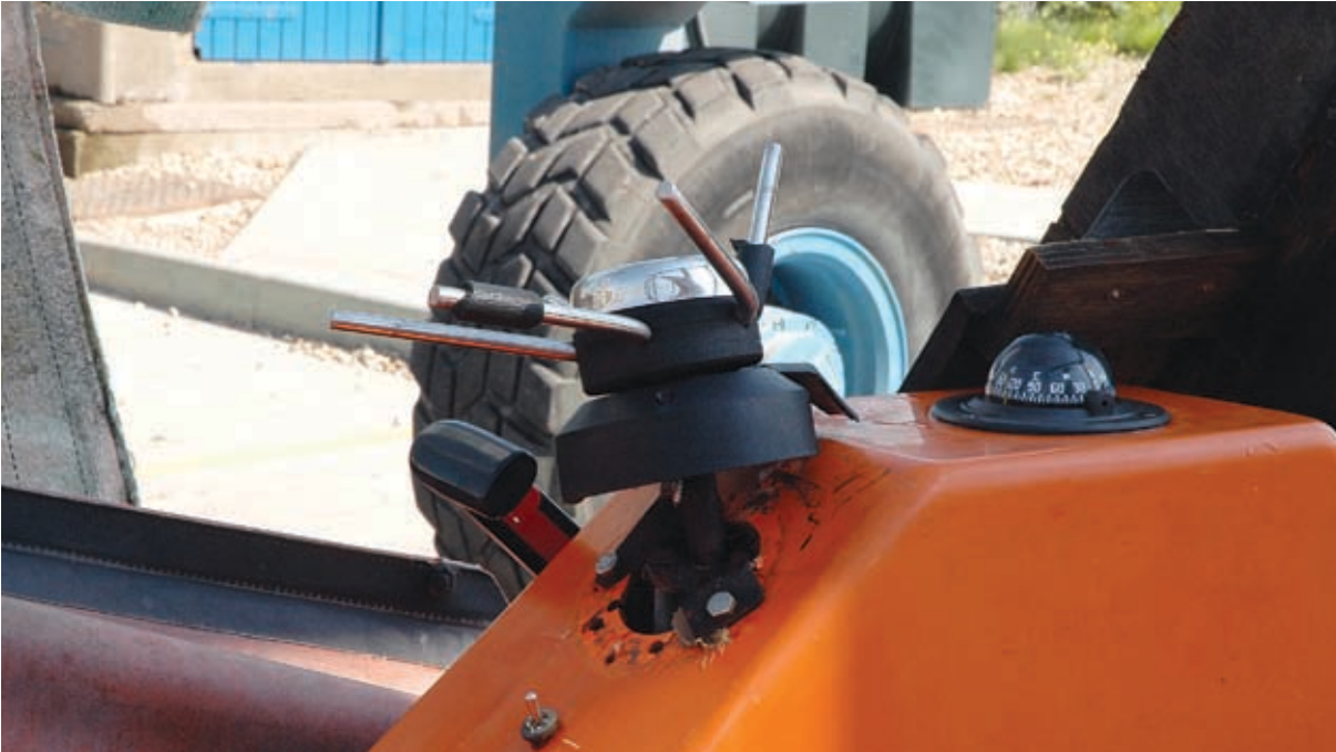
Damage to steering wheel following impact of the skipper
