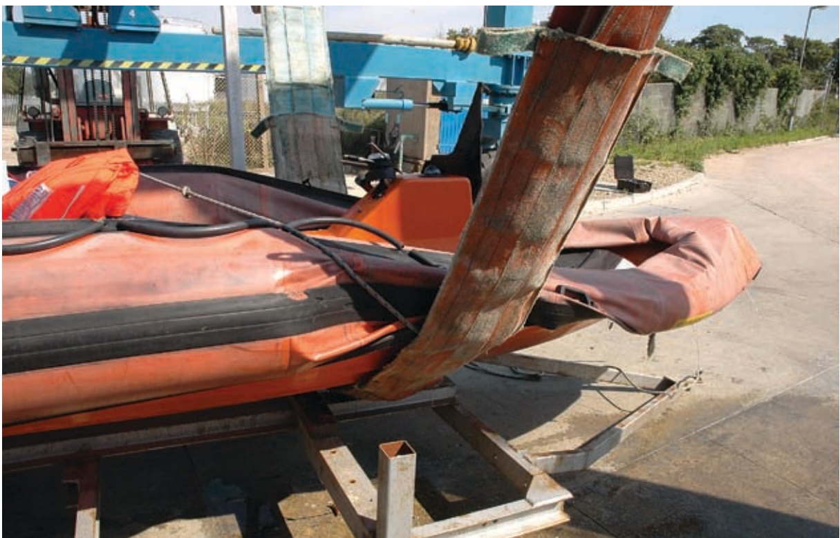
Recovered damaged RIB
