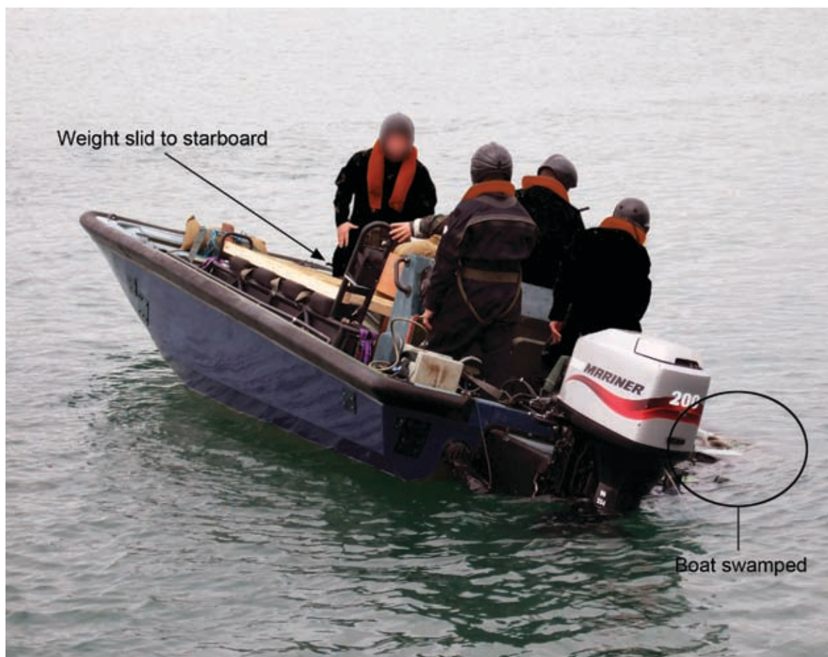
Capsizing trial illustrating weight shift and boat swamping
