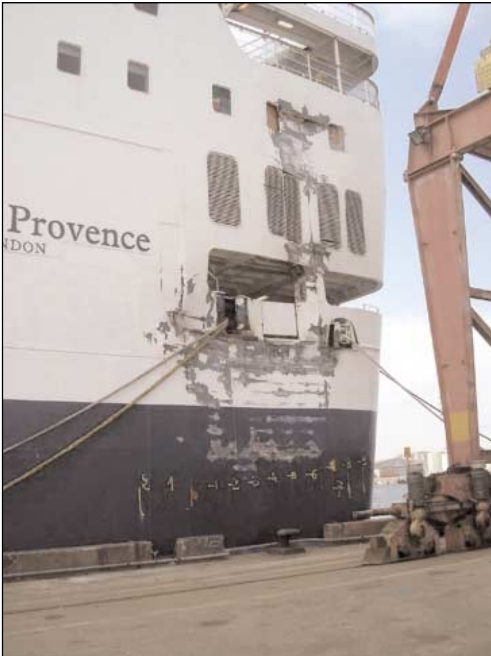
Damage to port quarter
