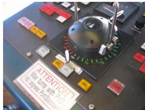
Control lever stoppers and signboard seen in stbd bridge wing, typical for all control positions.
