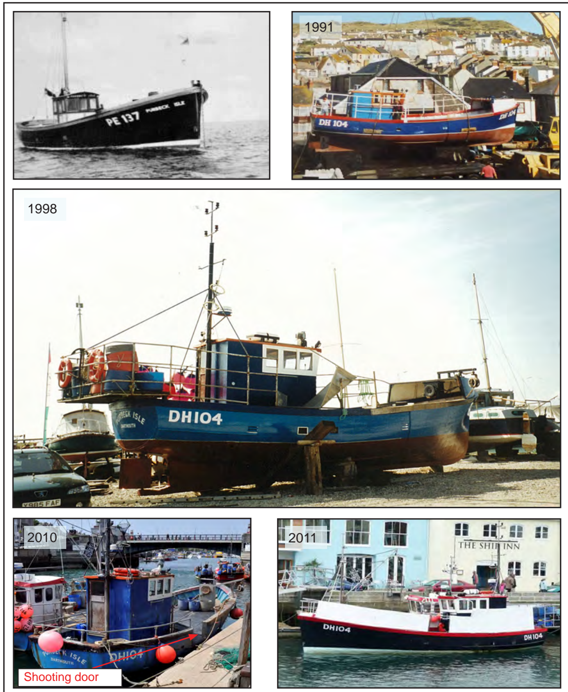
Figure 9: Purbeck Isle construction alterations and modifications
