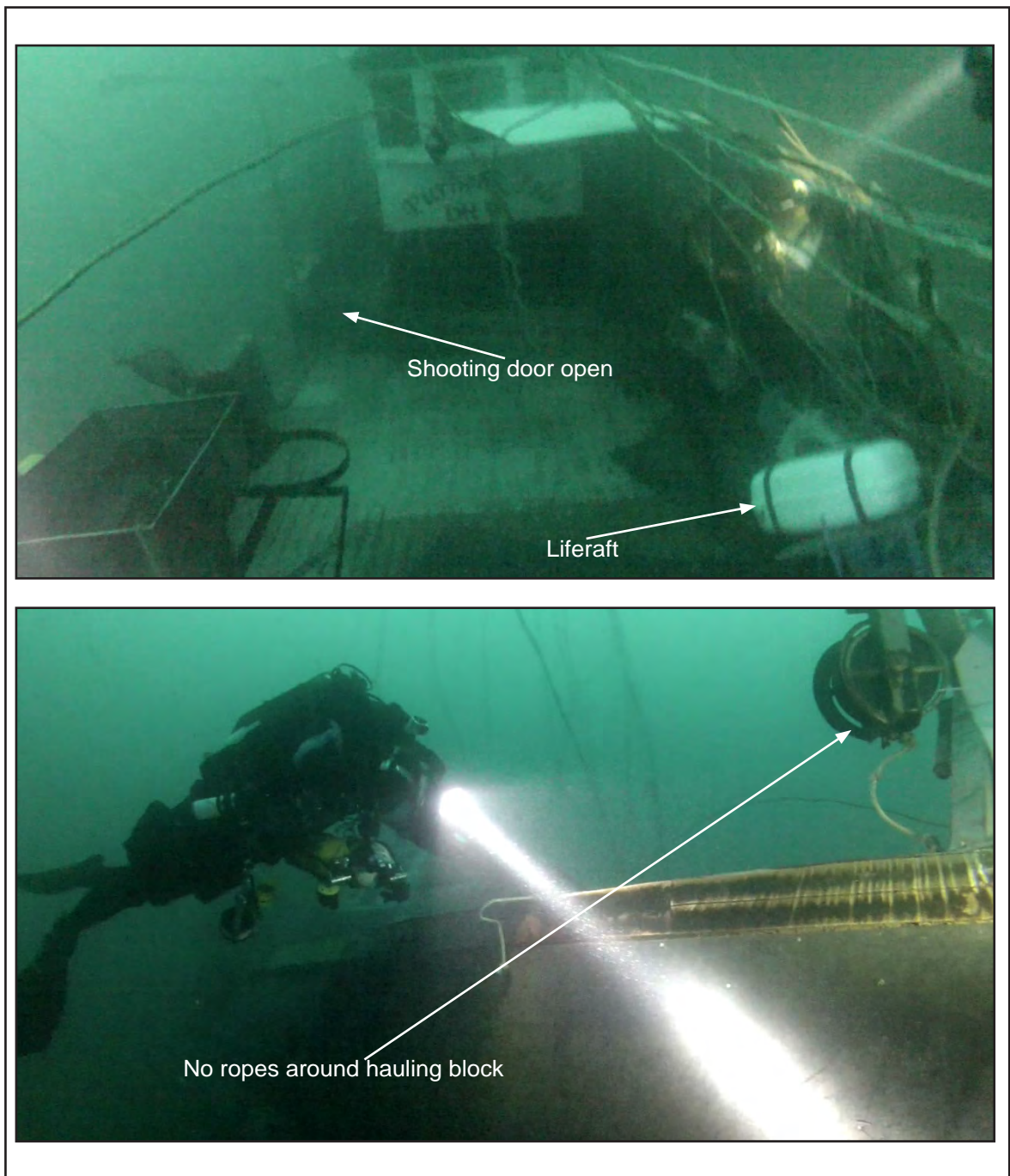
Figure 28: Dive one footage showing the deck forward of the wheelhouse
