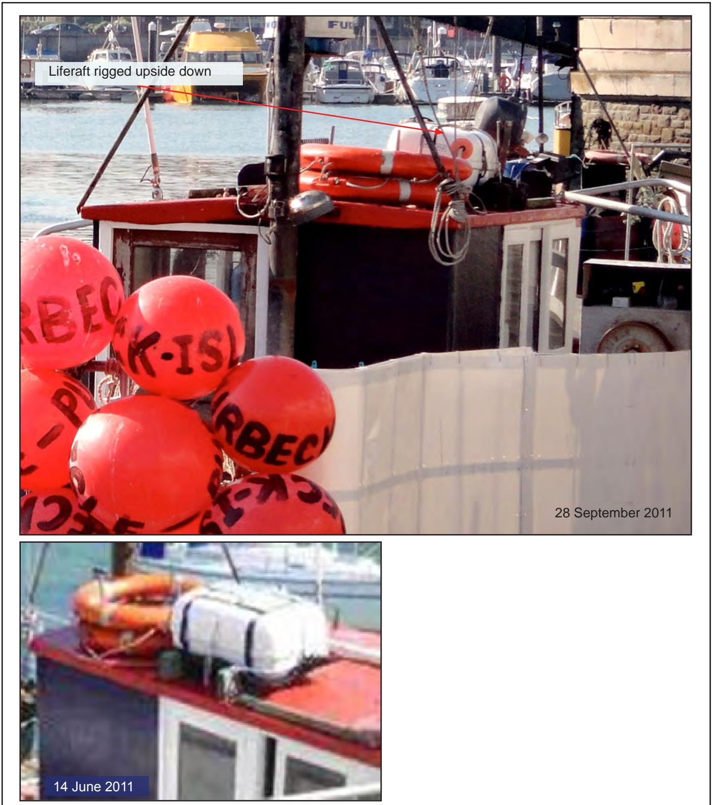
Figure 19: Liferaft lashed on wheelhouse roof
