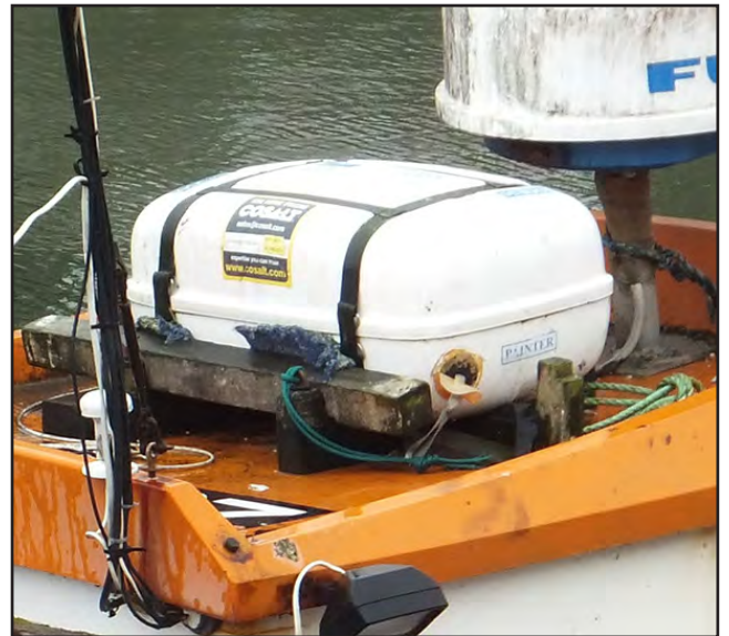
Liferaft rigged to float free but painter line is not attached to a HRU and raft does not fit in cradle
